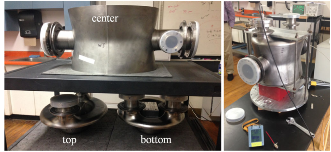
FIG. 6. (Left) Subassemblies for a DQW cavity. (Right) Clamped assembly of a DQW cavity.
