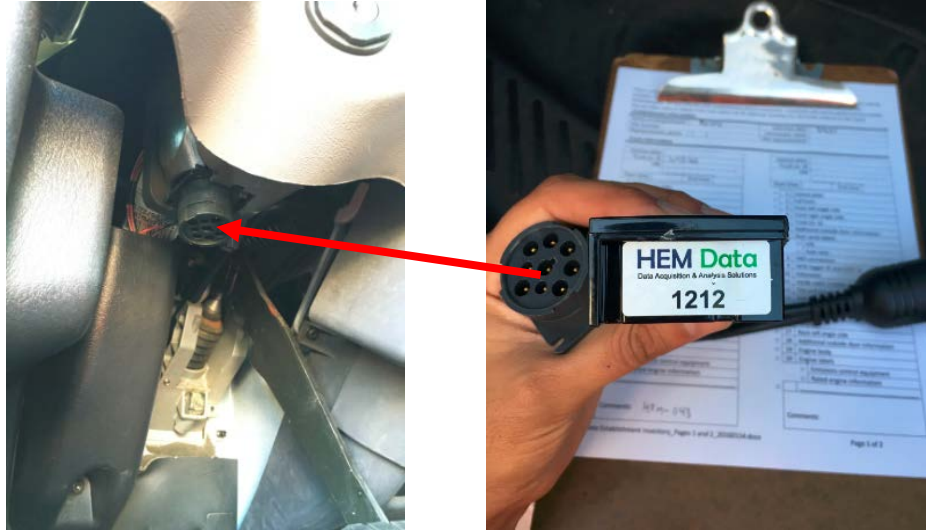
Figure 3-1. J1939 Mini Logger™ used in this research
