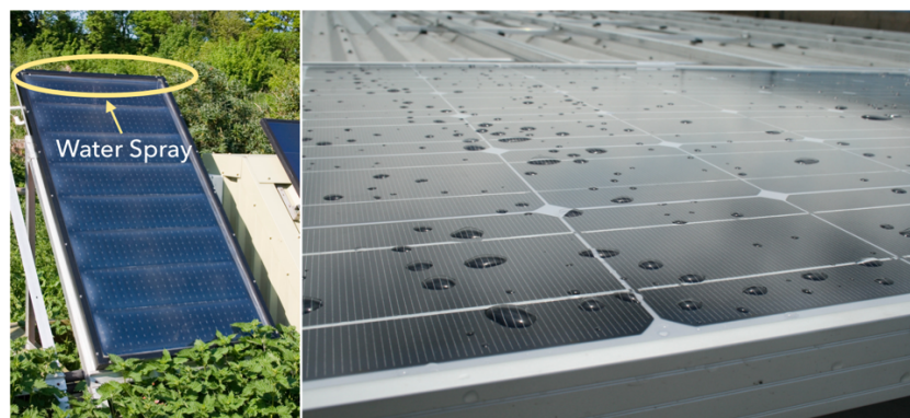
Figure 5. PV cells shown in use, with water cooling system attached on the top end of the set-up. Spraying of water on the surface of the cells helps cool them. (image courtesy: Dominic Alves)
