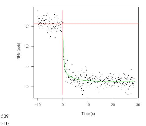
Fig 3. Time series of  $NH_3$  mixing ratio showing transient decay following removal of  $NH_3$  span gas from zero air flow to instrument inlet.
