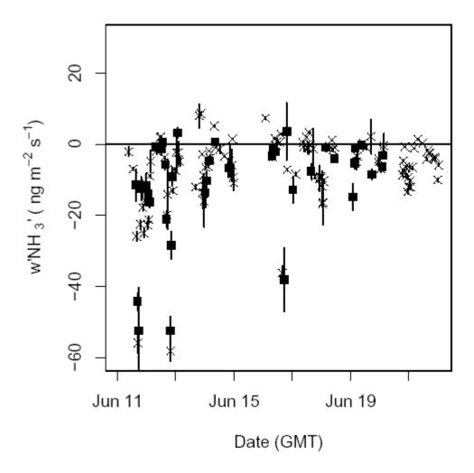
Figure 8. Eddy covariance measurement of NH<sub>3</sub> flux for all time points (crosses) and for those passing quality control criteria for use in calculating deposition velocities (filled squares).
