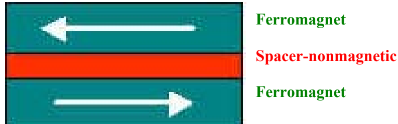
Fig-2 A GMR sandwich structure. Consisting of alternating magnetic and nonmagnetic metal layers. Layers.
