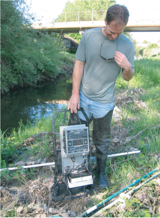
Rob Leidy from the EPA with the electro-shock box: this equipment provides the voltage needed to shock fish for two seconds, just enough time to net, bucket, and measure them.
