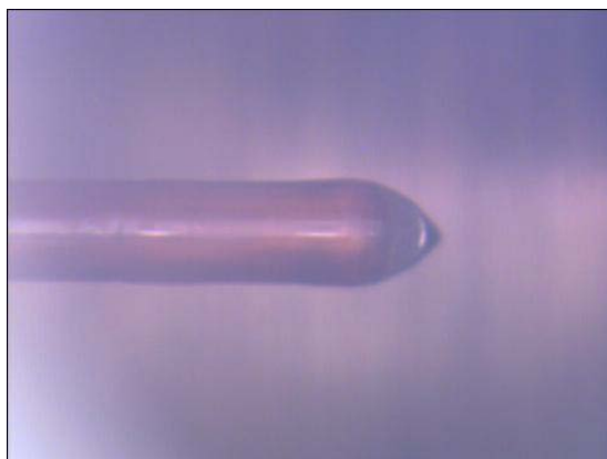
Figure 131. Electro spray formed in an externally-wet Silica emitter
