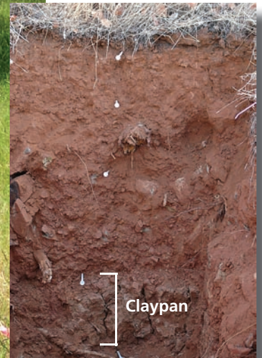
▲ The bracket shows an abrupt clay increase associated with the upper boundary of the claypan in a typical soil profile at SFREC.
