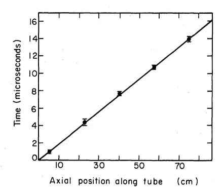
Fig. 5. Position of the ionization front vs time, as measured with radial current probes. The axial magnetic field was 15.7 kgauss, which resulted in a shorter transit time for the front than in the case shown in Fig. 3.
