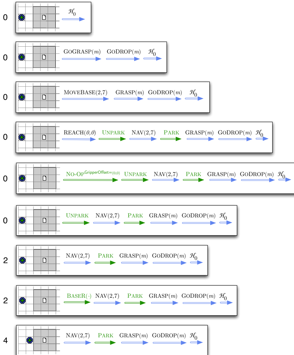
Figure 2.15: The first nine “hstates” encountered along an optimal solution for the discrete manipulation instance of Figure 1.1. Each hstate consists of a state (the relevant fragment of which is shown at left) paired with a sequence of actions remaining to do from this state. Each hstate is labeled with the total cost incurred to reach it, shown at left.
