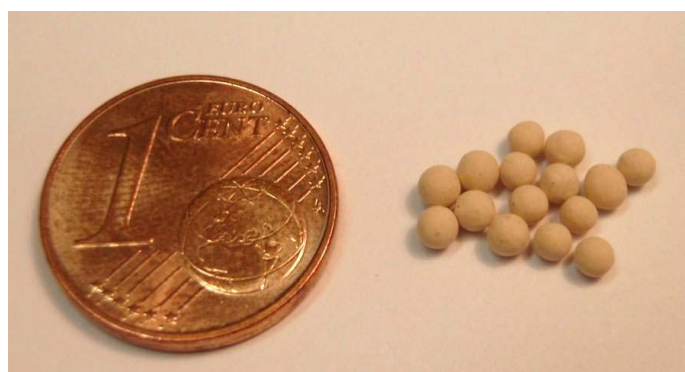
Figure 67: Photo of the ^{83}\text{Rb}/^{83\text{m}}\text{Kr} zeolite source. The zeolite is of type 5A, with spherical beads on average 2 mm in diameter.
