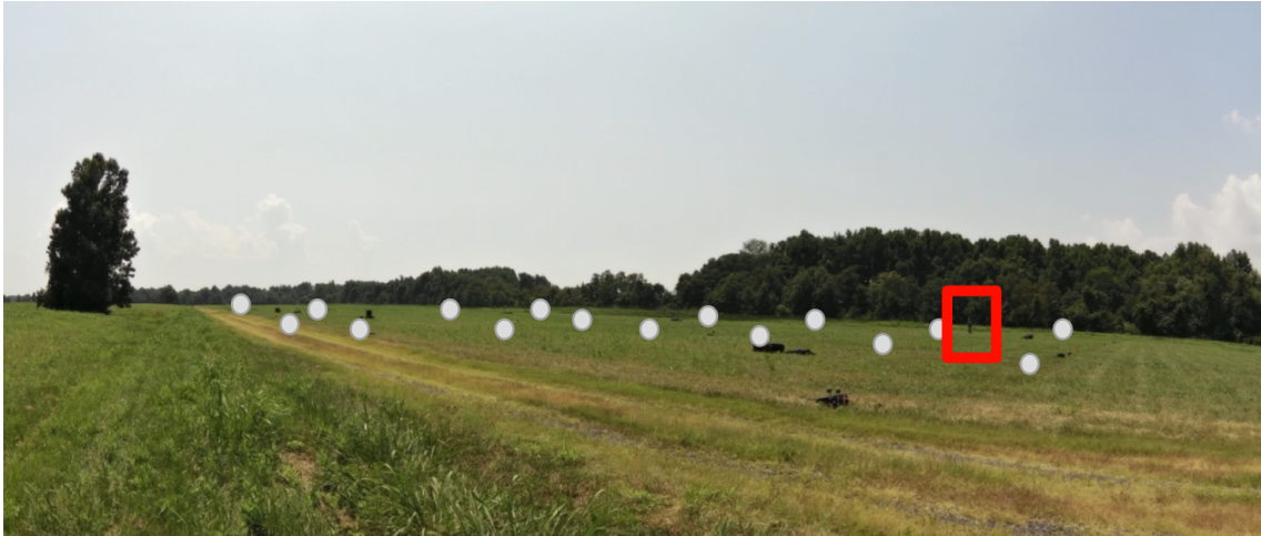
Figure 6.2: Wide field of view seen from one of the video cameras. White dots indicate the sensor locations and the red bounding box indicate the person’s location.
