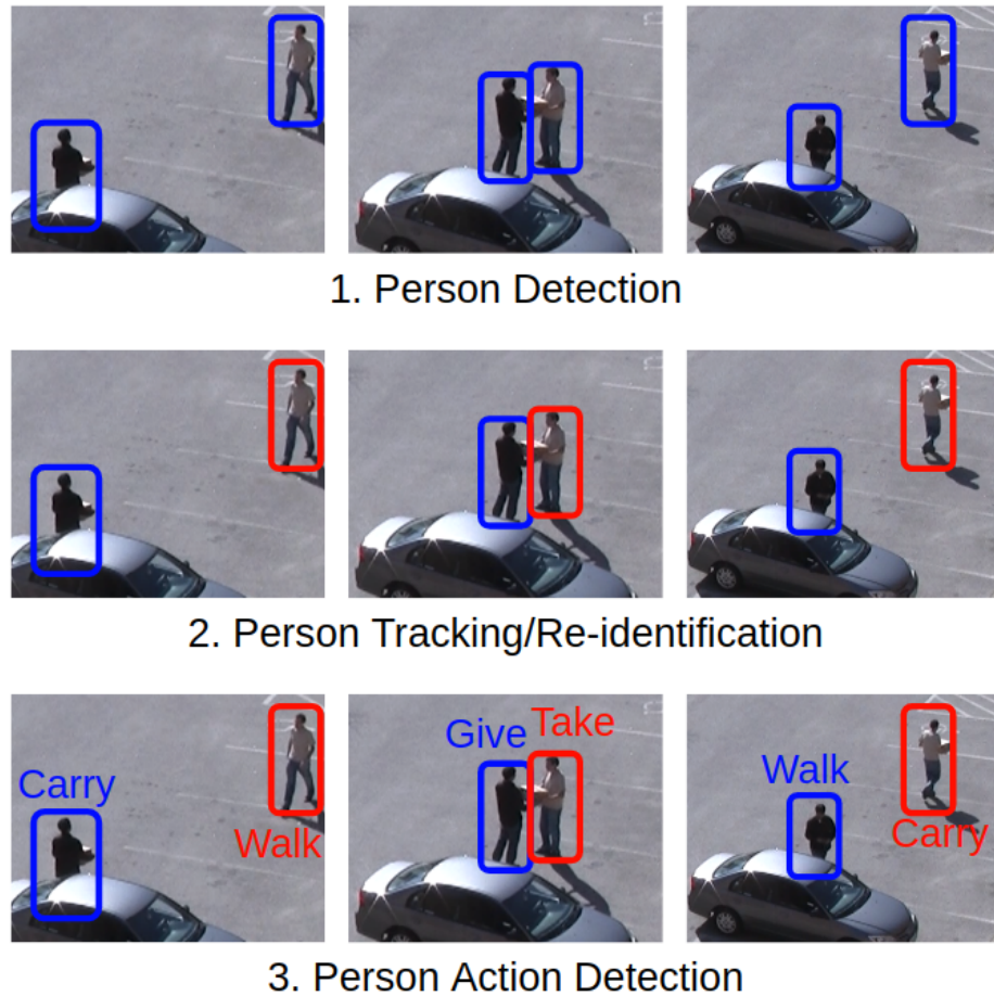
Figure 4.1: We combine 1) object detection models trained on object detection datasets, 2) trackers trained on human tracking problems and 3) action detection models trained on action detection datasets. Images are taken from VIRAT dataset [10]
