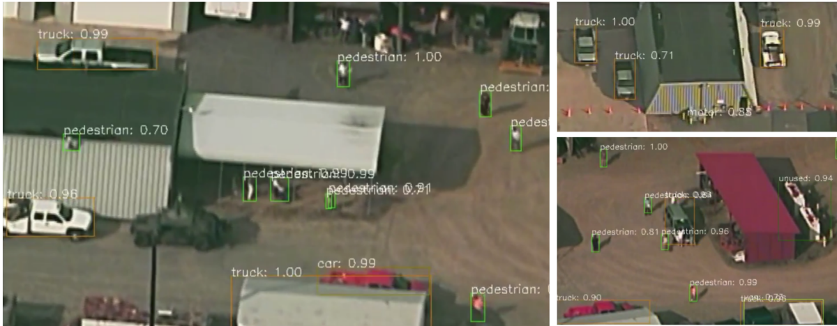
Figure 4.13: Qualitative results on images from VIRAT[10] Air dataset. Different colored boxes indicate different object classes. The altitude of the drone is significantly higher and the quality of the video is visibly worse than the Visdrone dataset. However, our model is still able to detect objects with some false positives and class confusion.
