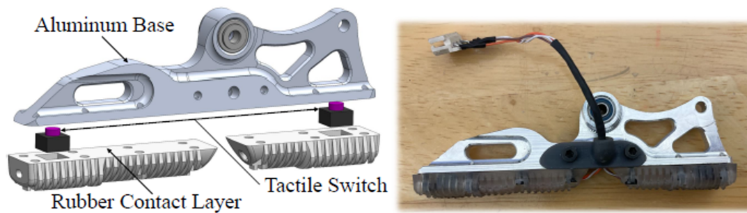
Figure 2.11: BRUCE contact sensing foot V2 design (left) and the actual hardware (right)
