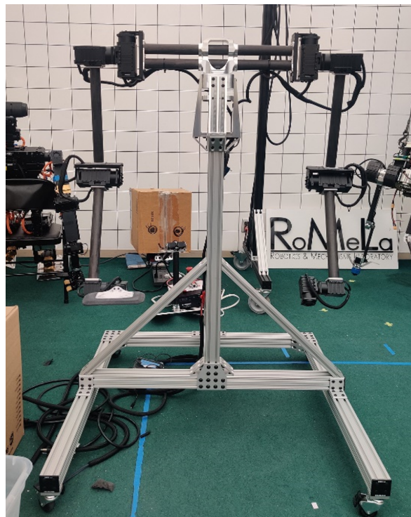
Figure 4.2: Prototype of YORI with traditional servo actuators [6]
