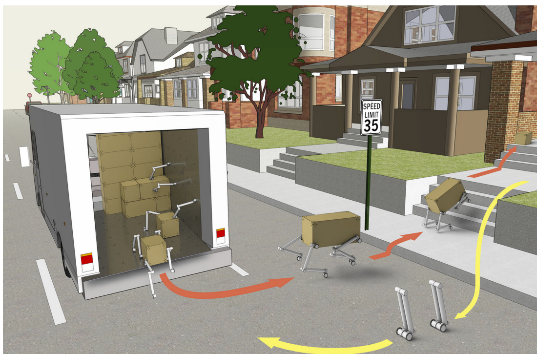
Figure A.1: LIMMS, or the Latching Intelligent Modular Mobility System, is designed for efficient last-mile delivery. While inside the delivery truck, LIMMS can pre-sort packages and queue them as needed, functioning like a manipulator by latching onto the truck walls to anchor itself. For package transport, four LIMMS units can attach to a box, using it as the central body to move the load like a quadruped robot. After delivery, each LIMMS unit switches to wheeled mode to return to the truck, ready for the next task. [8].
