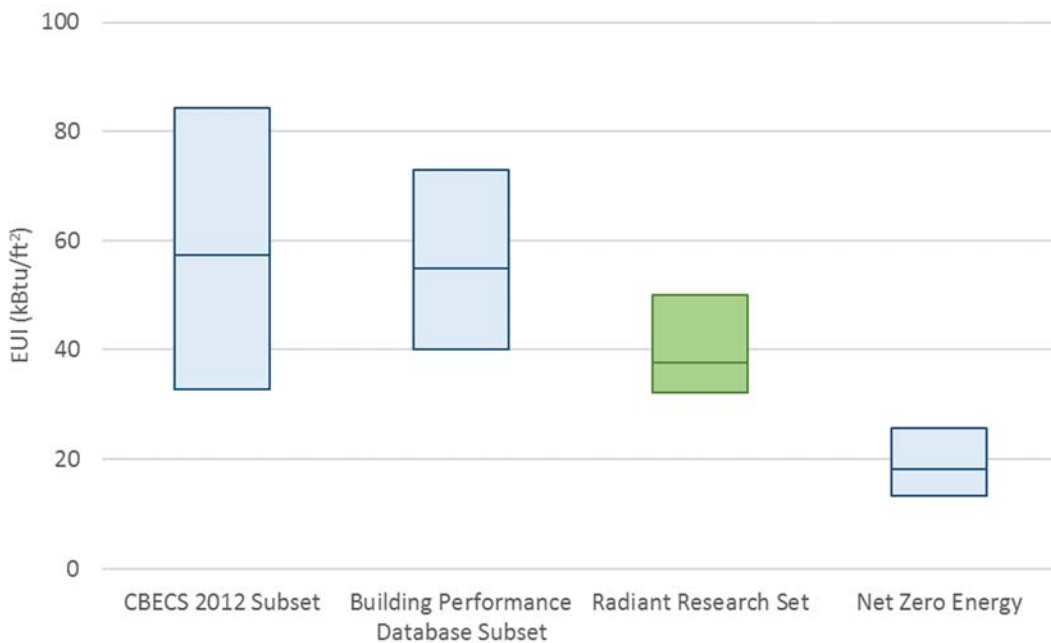
Figure 8: Box plot bounding 25 th and 75 th percentile EUIs of the research set and various benchmarks
