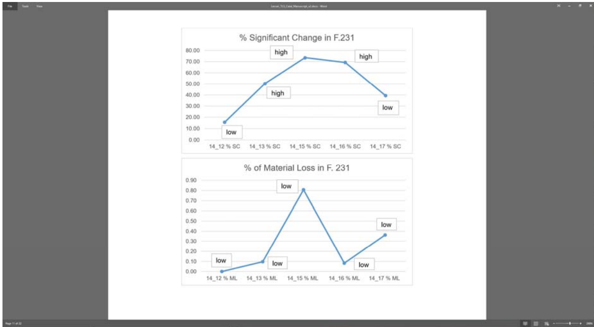
Fig. 8. % of Significant Change (SC) and % of Material Loss as detected in wall Feature 231 as detected in 2012-2017. High Significant Change > 40%, Low Significant Change < 40%. High % Material Loss > 1.3%, Low % Material Loss < 1.3%. Source: Arianna Campiani and Nicola Lercari
