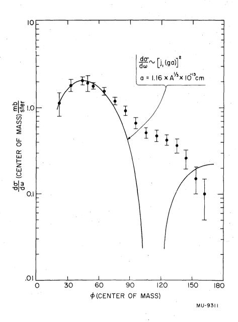
Fig. 11. Angular distribution of the differential cross section for the reaction  $p + C^{12} \rightarrow p' + C^{12*}$  (9.60 Mev) and the Austern, Butler, and McManus curve for  $\ell = 1$
