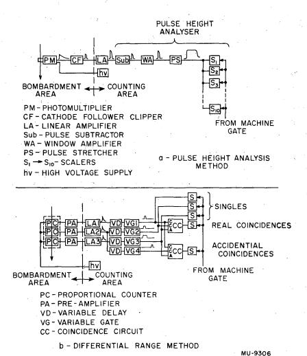
Fig. 3. Electronics, block diagram
