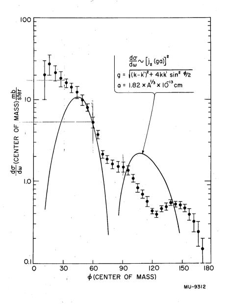
Fig. 10. Angular distribution of the differential cross section for the reaction  $p+C^{12}\to p'+C^{12*}$  (4.43 Mev) and the Austern, Butler, and McManus prediction
