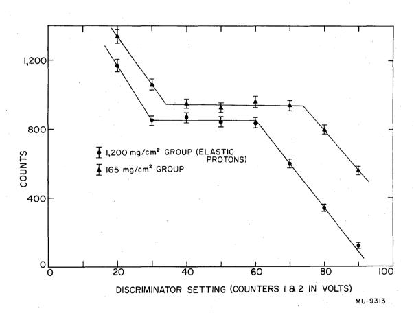
Fig. 8. Particle identification by dE/dx measurement
