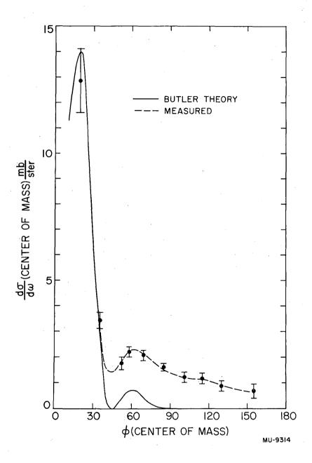
Fig. 12. Angular distribution of the differential cross section for the production of deuterons by the reaction  $p + C^{12} \rightarrow d + C^{11}$  and the Butler Theory prediction
