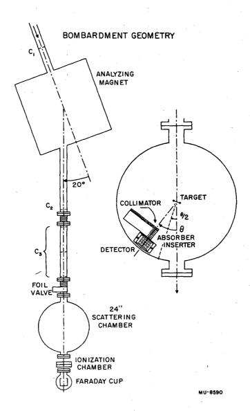
Fig. 2. Bombardment geometry
