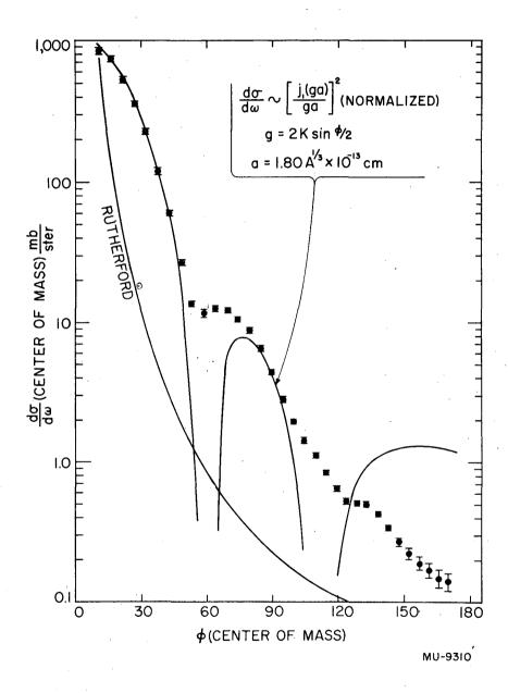
Fig. 9. Angular distribution of the differential cross section for elastic scattering of protons from  $C^{12}$  at 31 Mev (lab) and the Born approximation prediction
