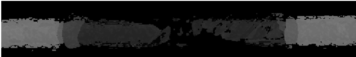
Figure 3.9. Example UT C-scan for cap impacted specimen S4C3 (47.1 J). Scanning captures the damage length but otherwise fails to capture many of the primary damage features due to curvature.
