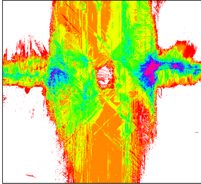
Figure 5.24. Map of delaminations and ply damage for specimen S4C2 color coded by the number of damage features in that region. The horizontal band of damage observed here is strongly associated with fiber damage and delamination traveling down the web.
