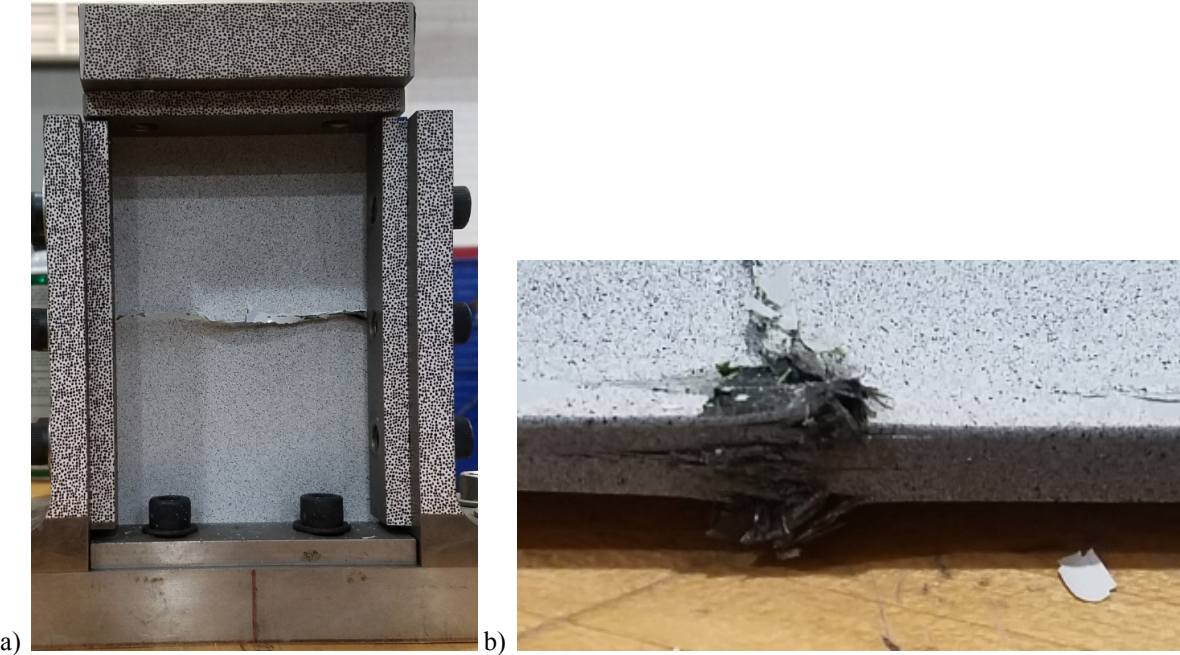
Figure 2.8. a) Specimen TC-24-31-1 in fixture post-failure. b) Image of brooming failure-
