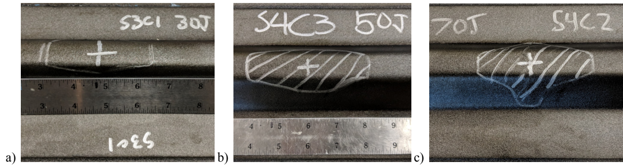
Figure 3.6. Handheld A-scan measurement of impact damage extent for cap impact case. a) Specimen S3C1, 28.5 J impact case. b) Specimen S4C3, 47.1 J impact case. c) Specimen S4C2, 66.7 J impact case.
