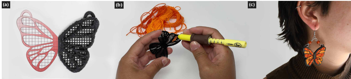
Figure 5.9: PunchPrint supports the creation of programmable and robust 3D-printed foundation textiles that are compatible with punch needle crafting. We present a design tool and fabrication workflow that reduces labor while supporting the production of detailed composite artifacts. Here we show how PunchPrint enables crafting small detailed designs. (a) We provide a parametric design interface for fabricating a flexible, filament-based textile substrate with design guides and hooks to facilitate assembly; (b) The craftsperson inserts fiber elements using standard punch needle embroidery methods on the 3D-printed foundation fabric; (c) The assembled final artifact with earring hooks and beads.
