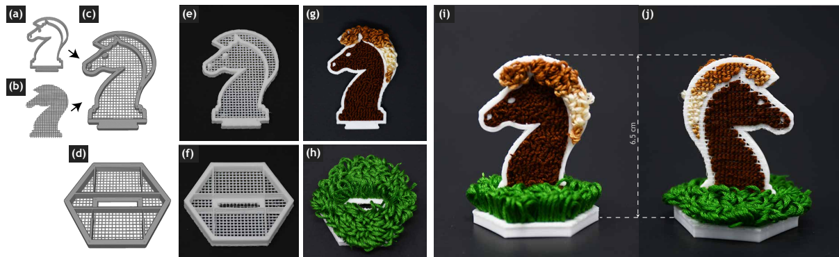
Figure 5.10: PunchPrint design workflow enables integration of our fabric method and complex geometry sliced with commercial slicers in the same print. It also creates an opportunity in assembling punched pieces together using press fit methods: (a) Surrounding geometry sliced with Cura; (b) our fabric generated in Grasshopper; (c) inserting the fabric GCode into sliced GCode results in a unified form; (d) the same procedure as in (a)-(b) repeated for the base of knight; (e) fabricated and (g) punched knight piece; (f) fabricated and (h) punched base piece; (i) the looped and (j) flat sides of the final artifact (6.5 cm).
