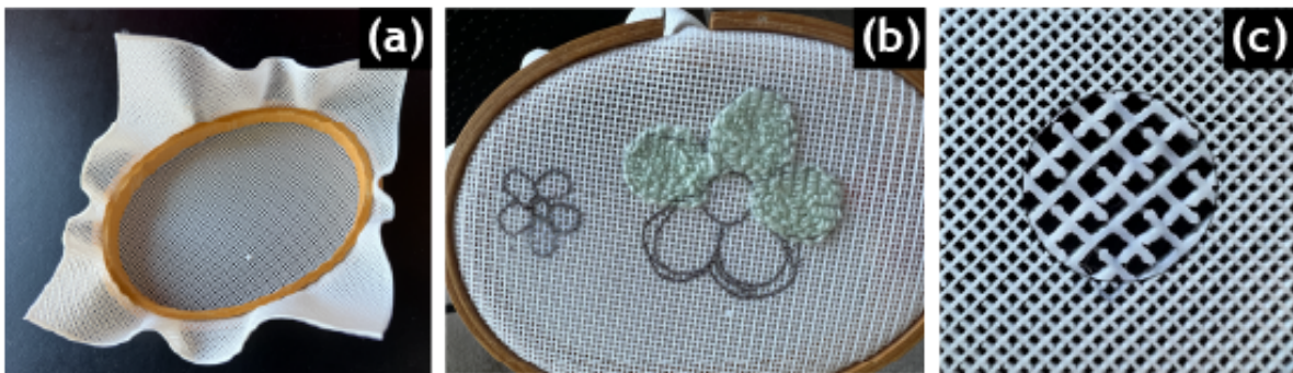
Figure 4.3: (a) The infill method offers a rapid way to produce TPU 3D-printed fabric. (b) Fabrics created with the grid or line infill pattern can be effectively used for punch needling. (c) The presence of weak points within these patterns results in the fabric breaking when subjected to the force of punching.
