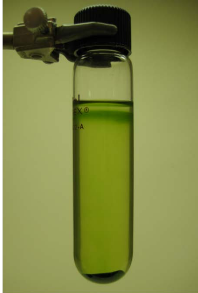
Figure 9. Centrifuged 50 mL tube of combined green layer and pellet from 2 previous 50 mL tubes with 20-25 mL of 480 mM sucrose + 5 mM \text{CaCl}_2 and a 3 mL PRML overlay. There were three distinct layers: a PRML upper layer, a green protoplast interface, and a sucrose + \text{CaCl}_2 underlayer. There was a large green pellet. Only the green protoplast interface was collected.
