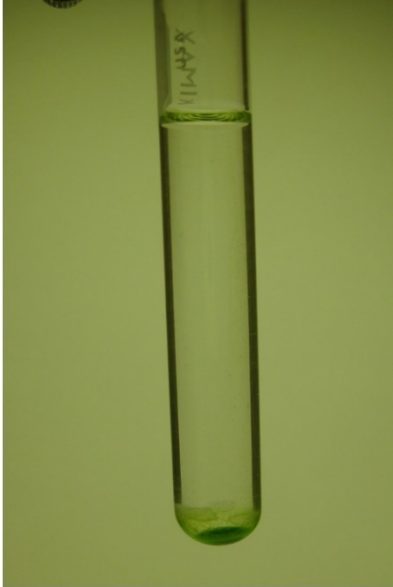
Figure 11. Centrifuged 13 x 100 mm tube of protoplast interface from the previous 16 x 125 mm tube, 3/4 full of PRML. In later experiments, PRML was replaced with MMM. Protoplasts should be at the bottom of the tube. The supernatant was discarded.
