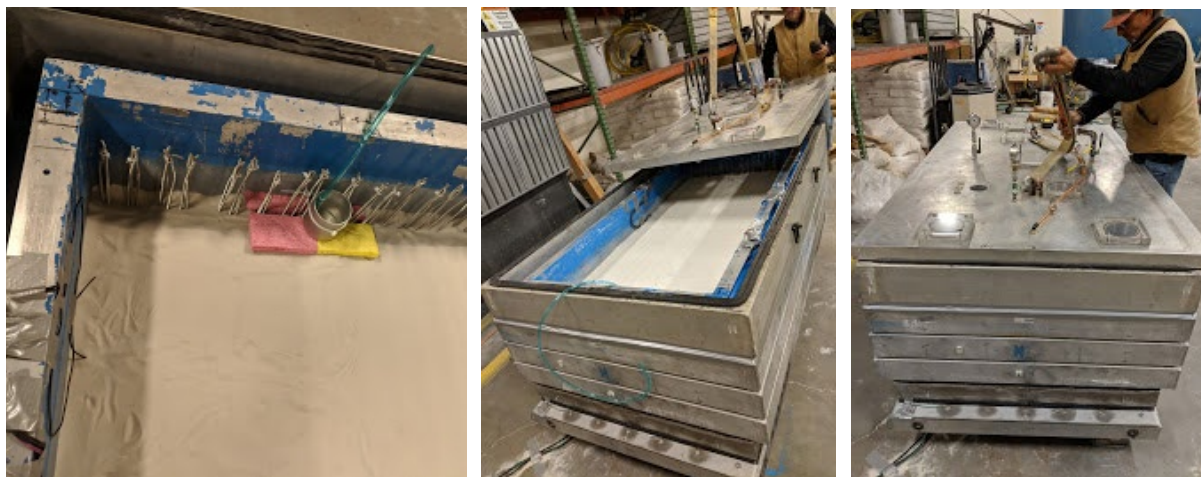
Figure 24. Preparation of the model for saturation.
