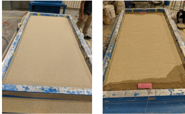
Figure 29. Model with Monterey sand layer.
