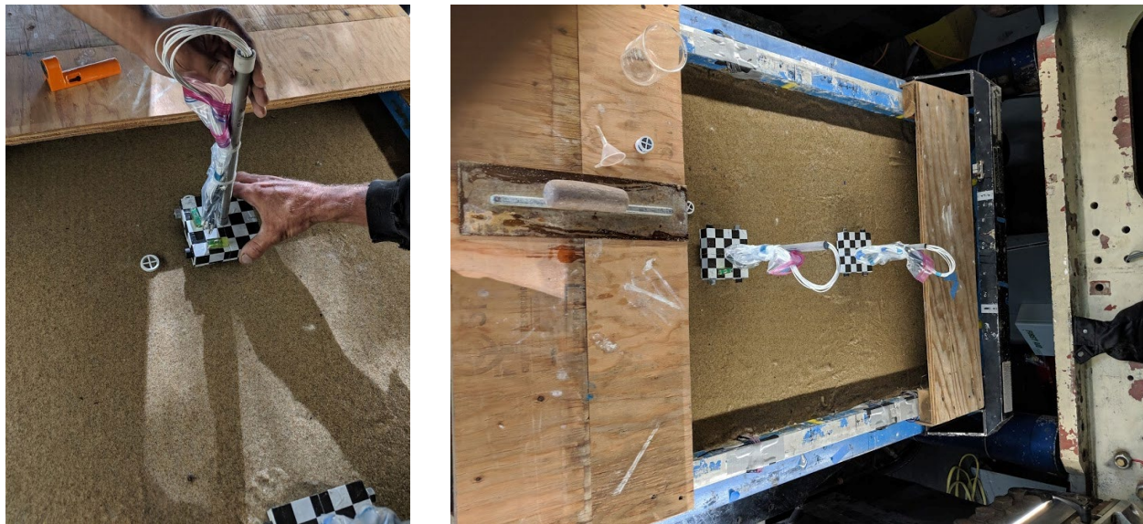
Figure 35. View of model with installed piles.
