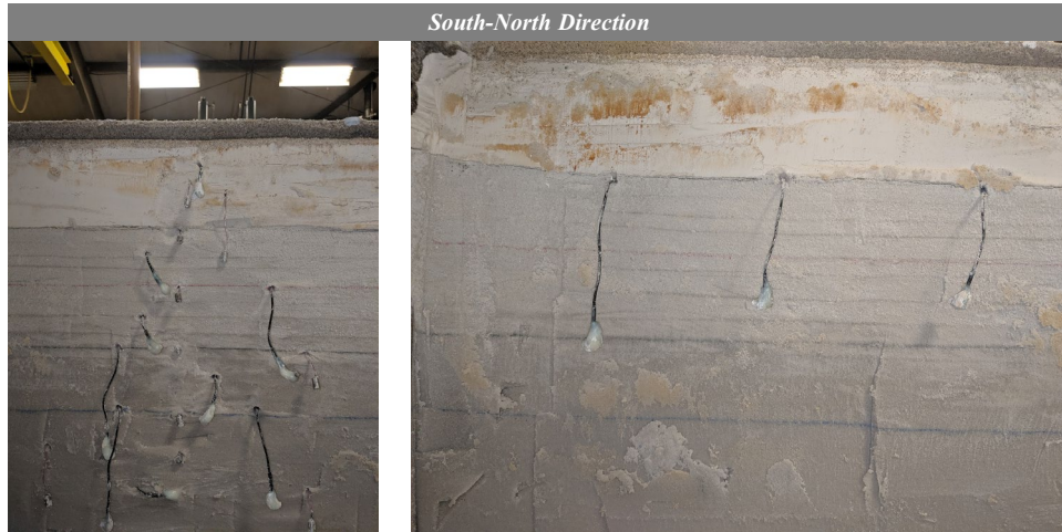
Figure 62. View of the sensors during model dissection.
