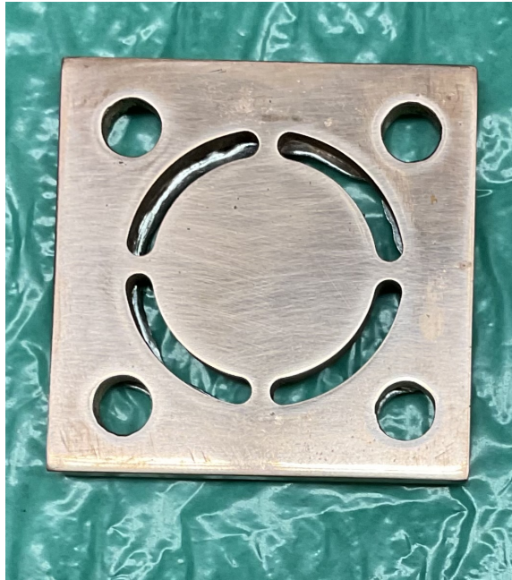
Figure 3.6: diffuser, the outer dimension of the plate is 1.5" x 1/5 " and the thickness is 1/8". The diffuser itself is 1" in diameter
