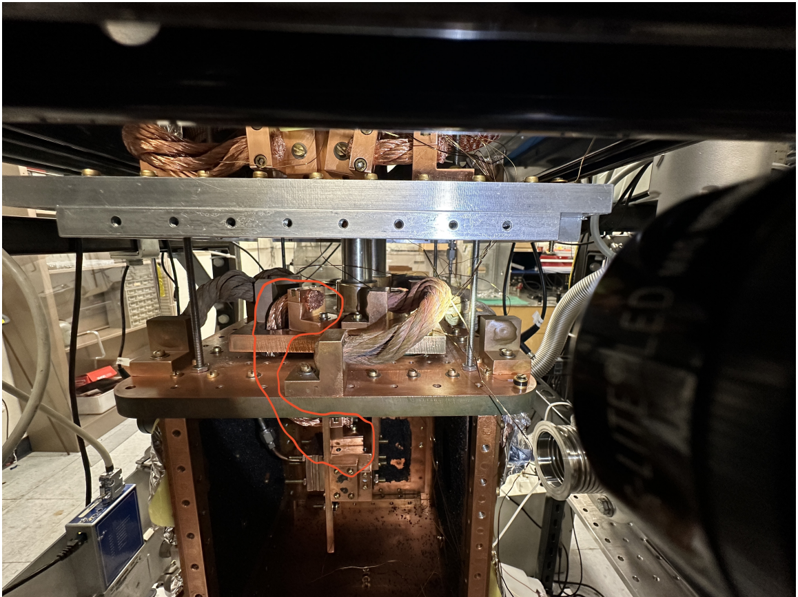
Figure 3.13: Direct thermal connection of the cell and the 4K pulse tube stage to increase cooling power for the cell
