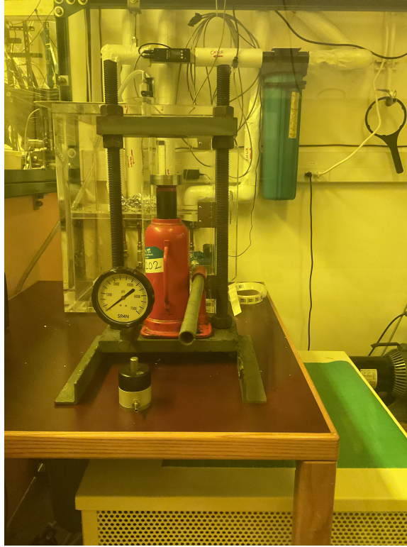
Figure 6.1: Hydraulic press and pellet dies used to make solid pellets of target. Typical pressure used is 6000psi and pressing time used to be 1 minute. However, we found pressing for 10 minutes increase the solid density of pellets and increase ablation yield.
