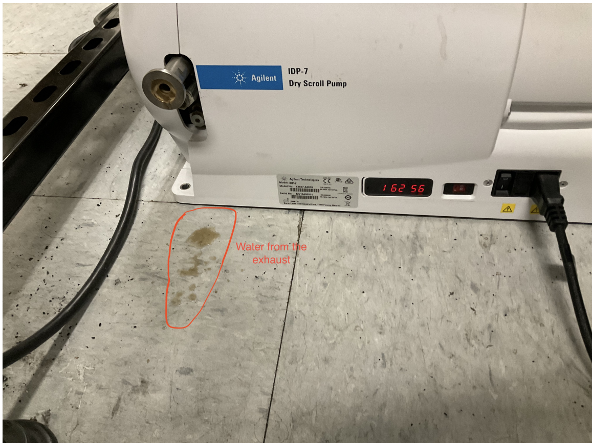
Figure 3.15: The IDP scroll pumps tends to accumulate water overtime and pumping efficiency decreases that causes the pressure to be one order of magnitude higher than working pressures.
