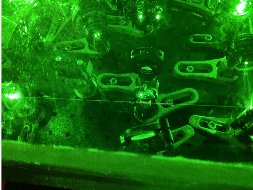
Figure 4.4: After installing a plastic box protection with dry air environment inside, clear beam of green light can be seen with no visible dust around
