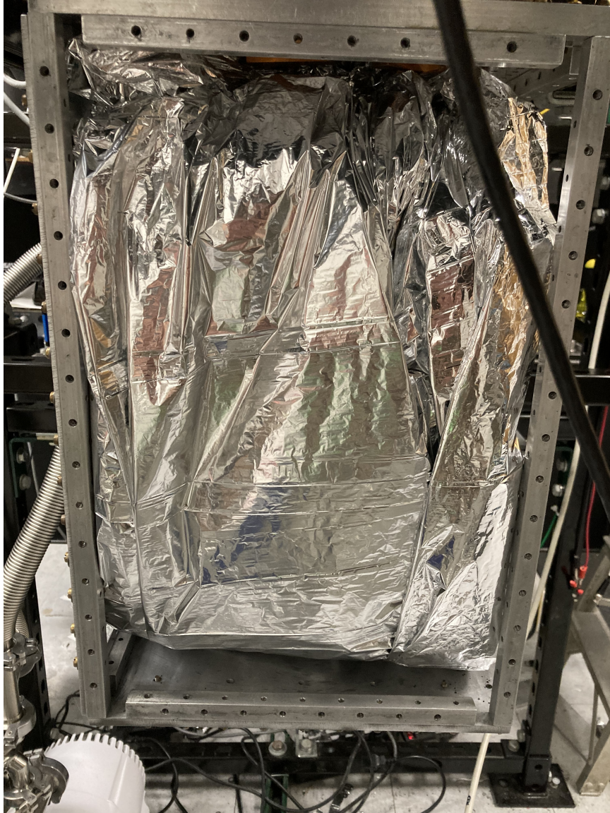
Figure 3.10: Super-insulation made of multiple layers of thin aluminum sheets to further reduce black-body radiation
