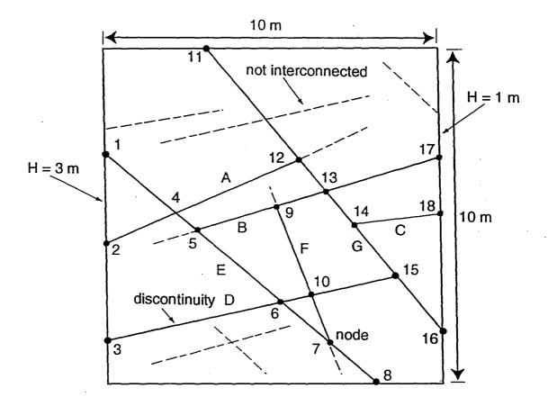
Fig. 2. Fracture network used in the saturated flow simulations conducted by Priest (1993). The left and right faces are held at uniform (but different) potentials, and the top to bottom faces have a linear potential gradient imposed along their lengths.
