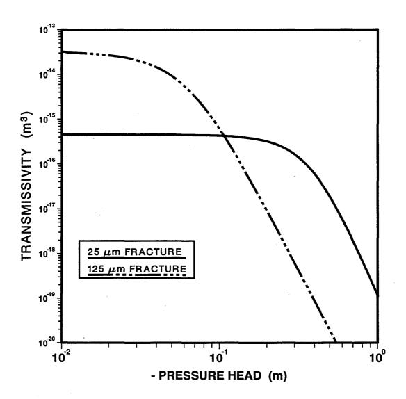
Fig. 4. Hydraulic conductivity functions for the two types of fractures used in the network shown in Fig. 2. The subvertical set of fractures have a mean aperture of  $125\,\mu m$ , and the subhorizontal set have a mean aperture of  $25\,\mu m$ .
