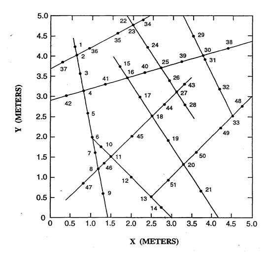
Fig. 3. Fracture network used in unsaturated flow simulations conducted by Kwicklis and Healy (1993). The top and bottom faces are held at the same pressure, so that the fluid flows from top to bottom due to gravity; the lateral sides are assumed to be impermeable.
