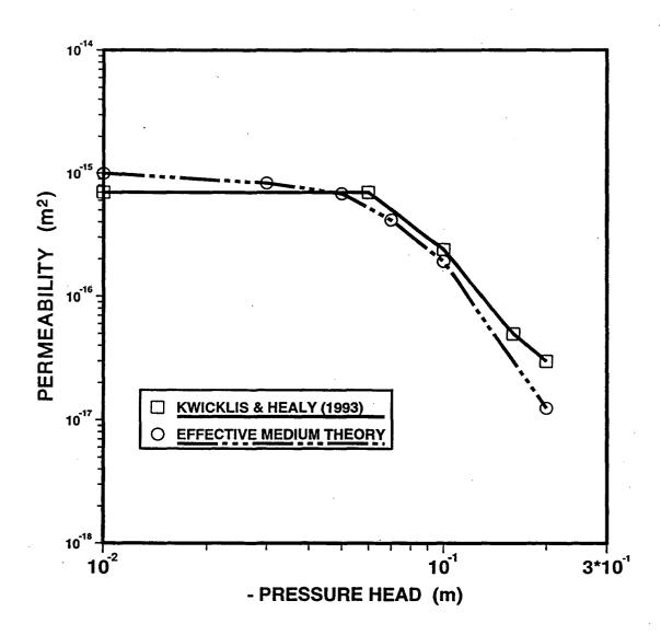
Fig. 5. Gridblock-scale hydraulic conductivity of the fracture network shown in Fig. 2, as a function of hydraulic potential, as calculated by numerical solution of the flow equations, and by using the proposed upscaling procedure.
