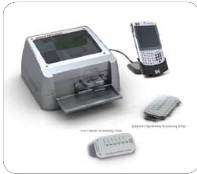
FIGURE 8. The UCLA oral fluid nansosensor test (OFNASET): Showing two chips, one for oral cancer screening and one for Sjögren syndrome screening ( courtesy of Dr. David Wong ).
