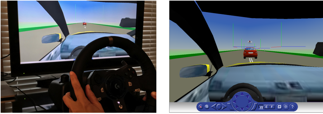
Figure 6.6: Vehicle dynamics virtualization testbed used in the evaluation study .
