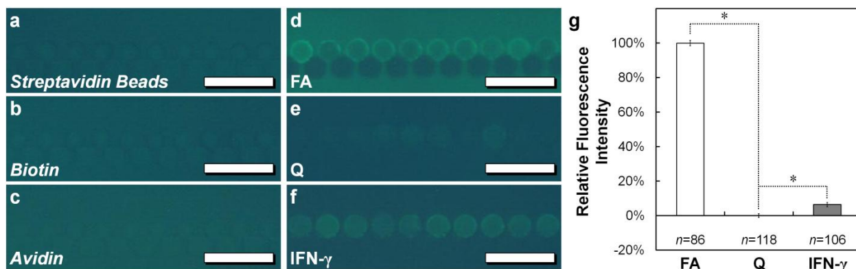
Figure 3.18 Experimental results for IFN- \gamma detection via an aptamer-based sandwich assay in the MPP System. (a-f) Fluorescence micrographs of arrayed 15 \mu\text{m} diameter microbeads after each step of the aptamer-based sandwich assay (see Fig. 3.4 ). Scale Bars = 50 \mu\text{m} . (g) Average relative fluorescence intensities ( RFIs ) of arrayed microbeads after mixing with the FA, Q, and IFN- \gamma solutions. RFIs were quantified using Equation 3.5 . Error Bars denote s.e.m.; * denotes p < 0.0005 statistically significant differences.
