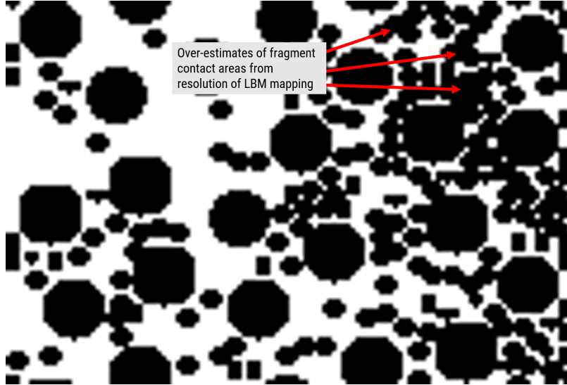
Figure 6.41: Over-estimates of contact area of fragments contributes to higher heat conduction in LBM model than CFD-DEM.
