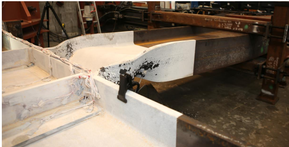
Figure 4.126 Specimen W2: East Beam Bottom Flange Lateral-Torsional Buckling at: -0.06 rad (1 st Cycle)
