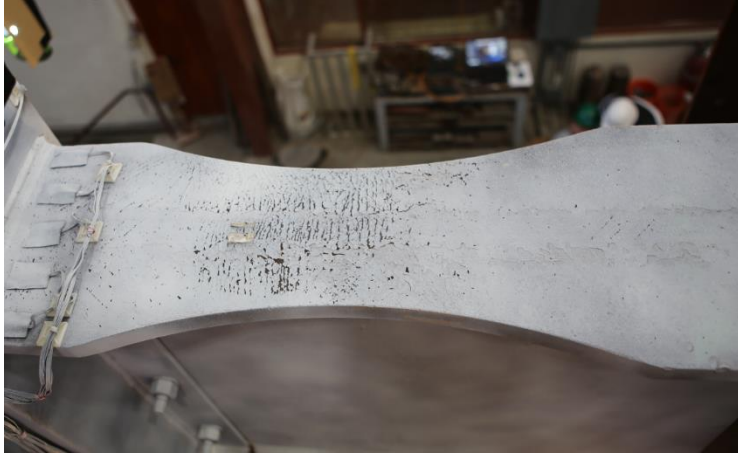
Figure 4.81 Specimen C7: Beam Top Flange Yielding at -0.015 rad (2 nd Cycle)
