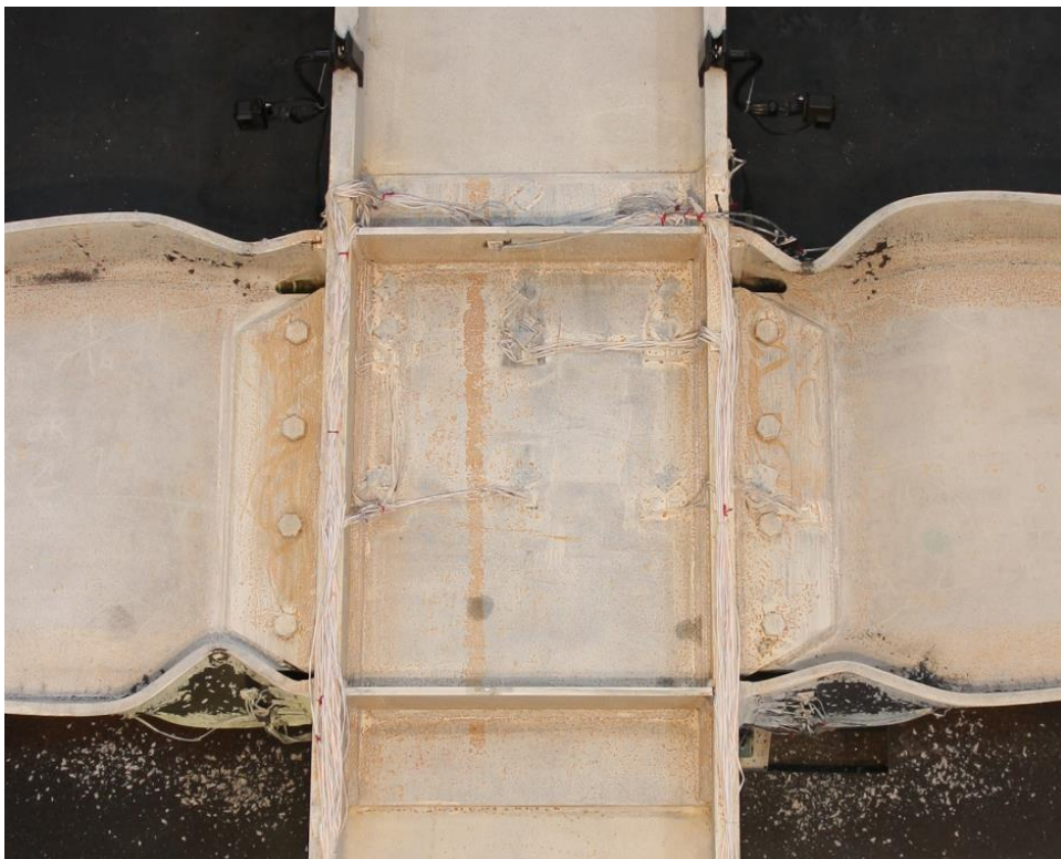
Figure 4.147 Specimen W3: Flange Local Buckling at -0.05 rad (1 st Cycle)
