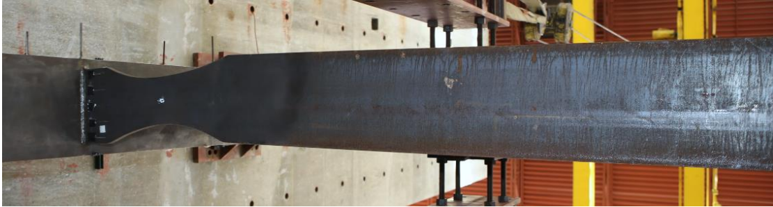
Figure 4.7 Specimen C3: Beam Lateral-Torsional Buckling (End of Test)
