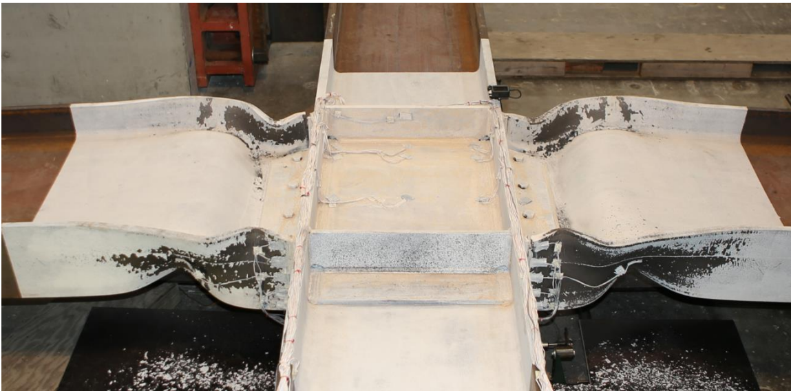
Figure 4.130 Specimen W2: Connection at End of Test
