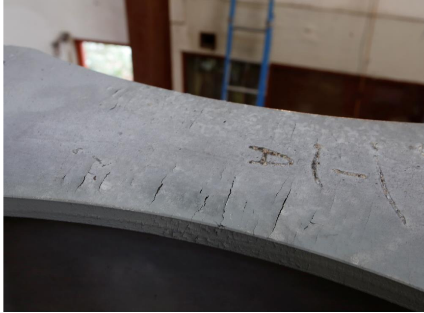
Figure 4.64 Specimen C6-G: Cracks in Galvanization Coating
