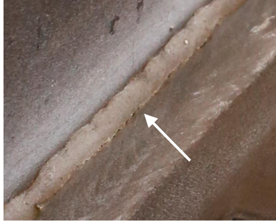
(b) Tearing at -0.03 rad (2 nd Cycle)
