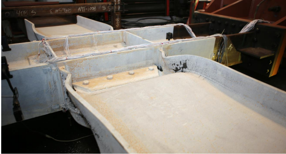
Figure 4.146 Specimen W3: Web Local Buckling at +0.05 rad (1 st Cycle)
