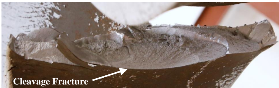
(b) Fracture Surface
