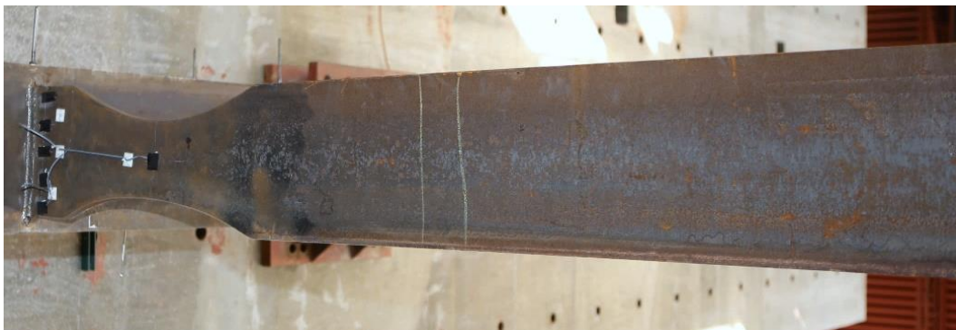
Figure 4.39 Specimen C5: Beam Lateral-Torsional Buckling (End of Test)
