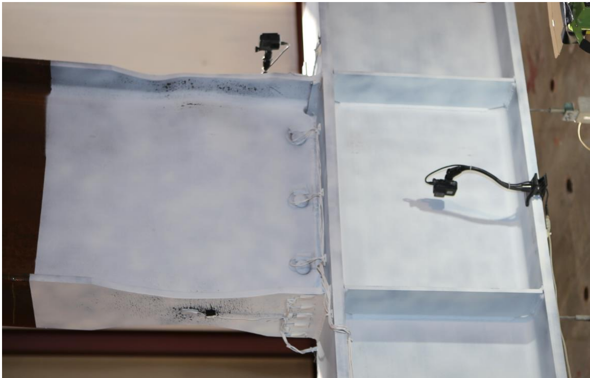
Figure 4.53 Specimen C6: Beam Web and Flange Local Buckling at +0.04 rad (2 nd Cycle)
