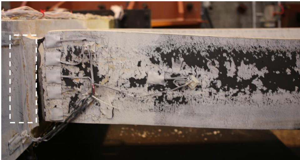
Figure 4.173 Specimen W4: East Beam Top Flange Fracture during First Excursion of -0.05 rad
