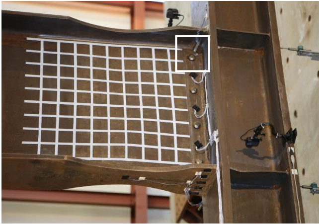
(a) Beam Web Buckling
