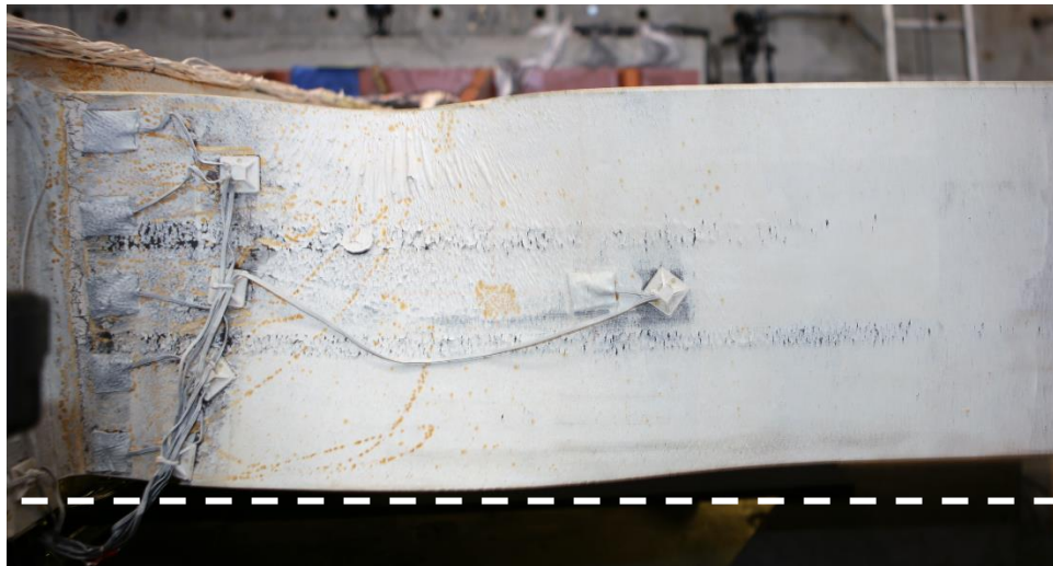
(a) East Beam Top Flange at +0.04 rad (2 nd Cycle)
