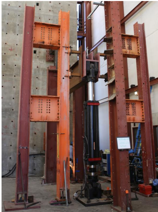
Figure 3.3 Lateral Bracing at Loading End (Phase 1)
