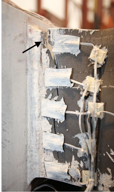
Figure 4.129 Specimen W2: West Beam Bottom Flange Fracture during Excursion to -0.06 rad (2 nd Cycle)
