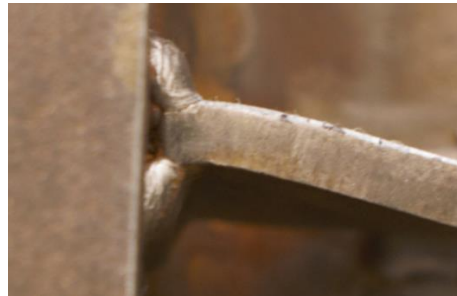
(b) Enlarged View of Weld
