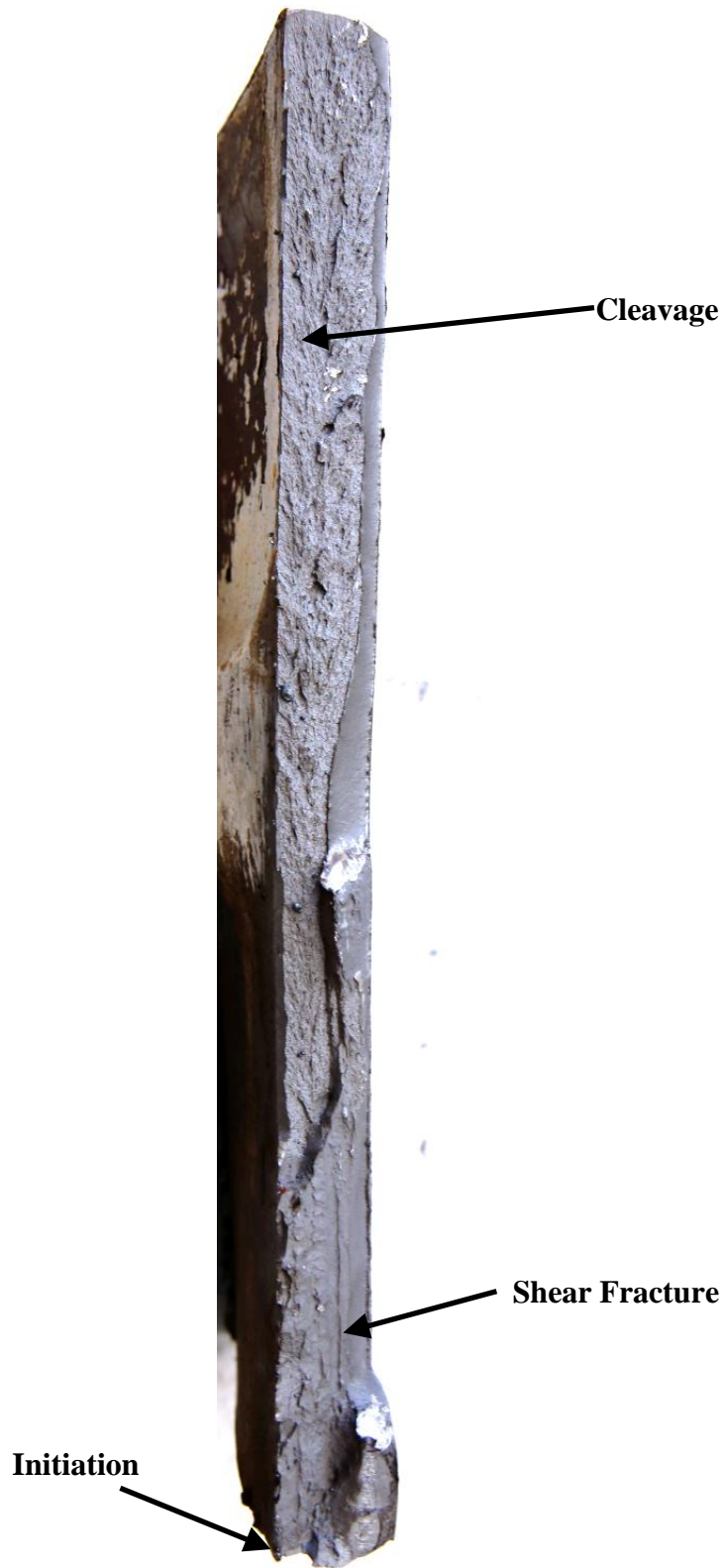
Figure 4.105 Specimen W1: East Beam Top Flange CJP Weld Fracture Surface
