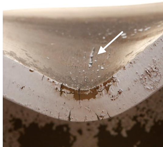
(b) Ductile Tearing
