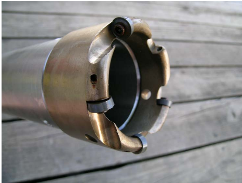
Figure 1-5. Core barrel. One carbide tooth is missing.
