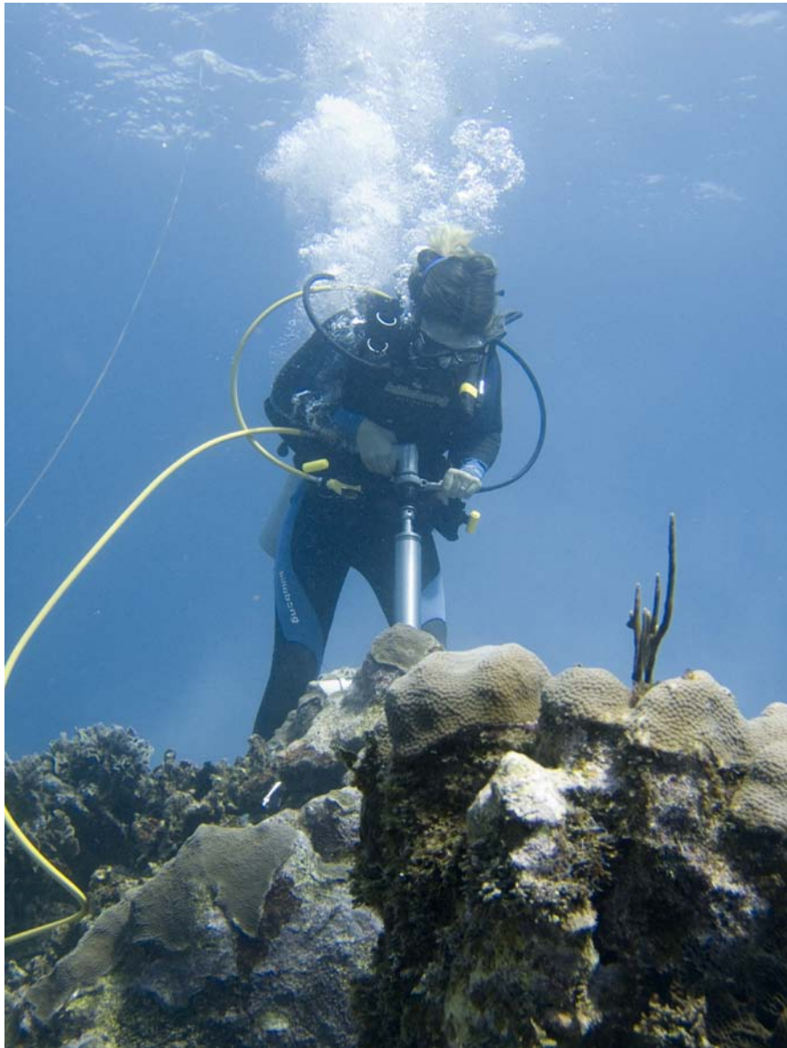
Figure 1-4. Drilling a coral core in Belize. Photo by Brad Erisman.
