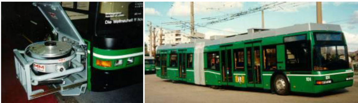
Figure II-6 Examples of Modern Transit Bus Flywheel Energy Storage Systems
