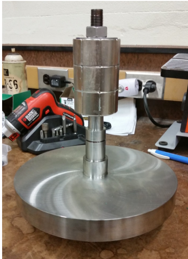
Figure III-34 Assembled INSTAR Rotor and Flywheel Shaft
