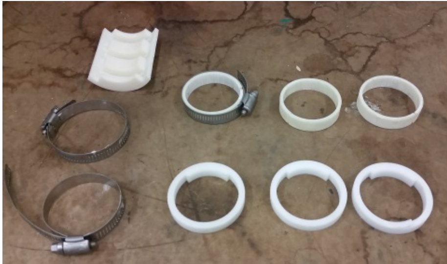
Figure III-35 3D Printed Rotor Assembly Jig
