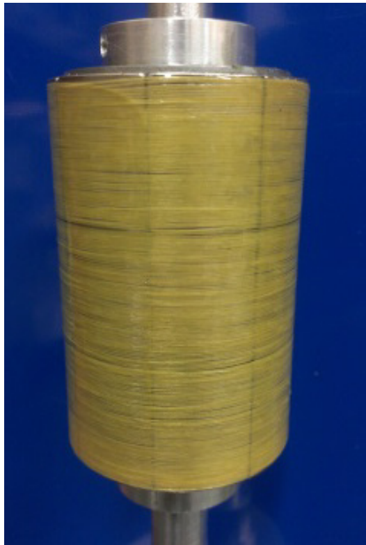
Figure III-39 Finished Rotor After Magnet Epoxy and Kevlar Wrap
