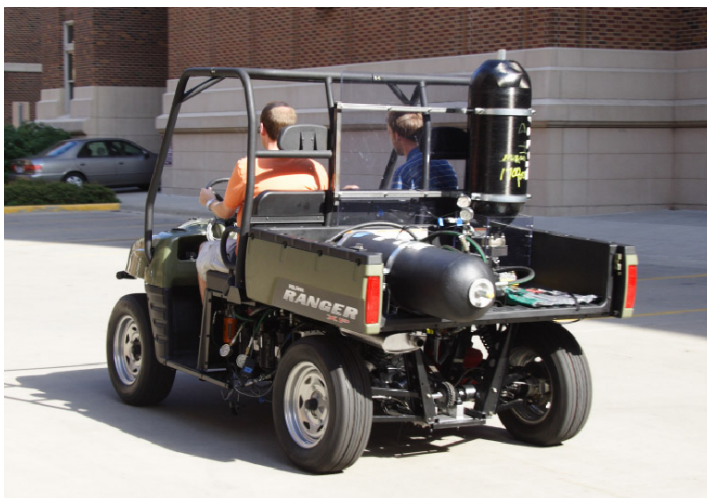
Figure II-7 Hydraulic Regenerative Braking Test Vehicle
