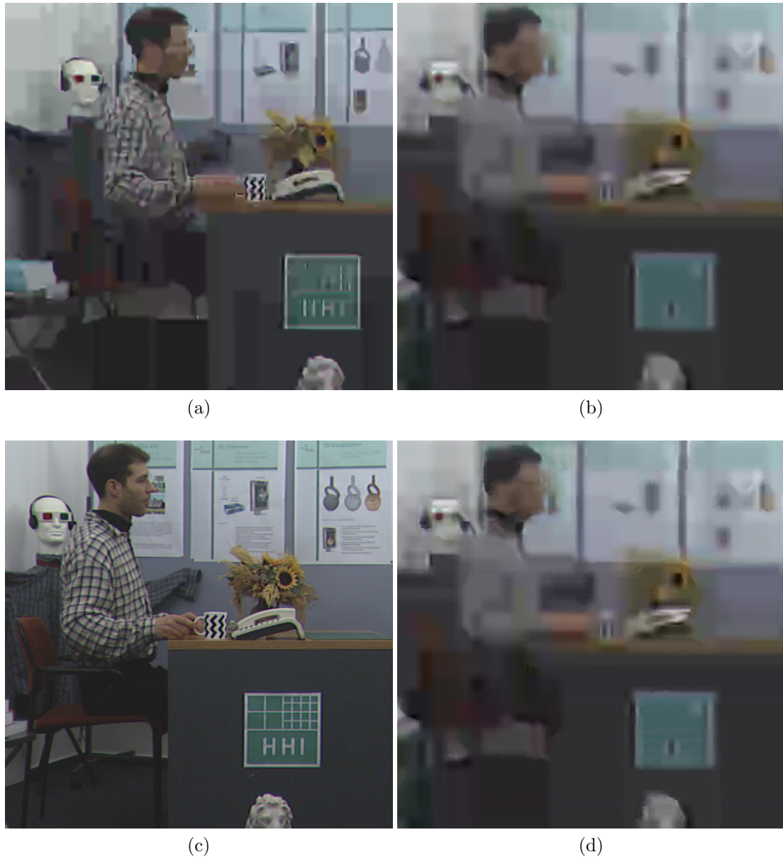
Figure 4.10: Sample image results from Book_Arrival sequence for QP = 50 . Images are 480 \times 480 cropped from frame 5 of sequence, top left pixel coordinate (row, column) = (125,150). (a) Reference (left) view (b) interpolated test (right) view (c) ground truth test view (d) super-resolution output of test view.
