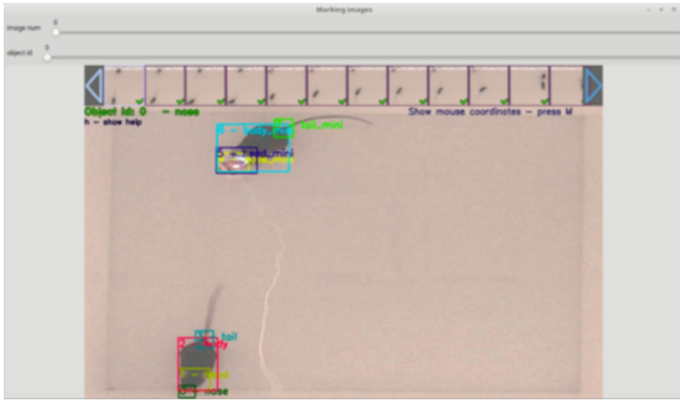
Figure 5: GUI of Yolo_Mark to label images in a format acceptable for Yolov3. Please click here to view a larger version of this figure.
