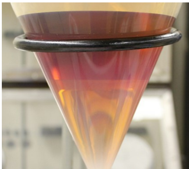
(a) Forward-extraction phase separation (TBP organic phase on top; \text{HNO}_3 aqueous phase on bottom).
