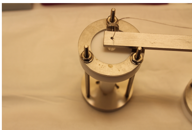
(b) The fully assembled cell with the anode wire suspended in the chimney.
