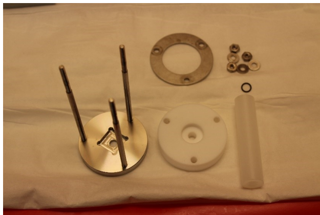
(a) Disassembled components of the cell (including the steel frame, plastic chimney Teflon cap, steel ring, screws and washers and o-ring).
