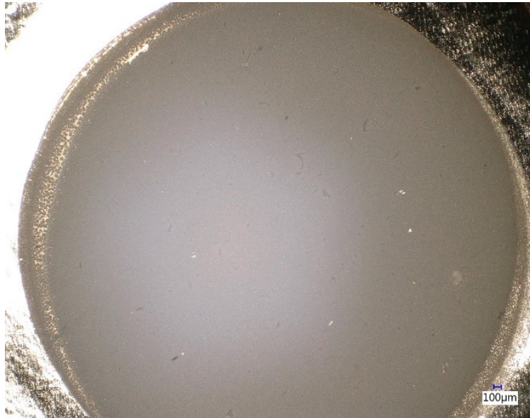
(a) ThO 2 ( 1410 \pm 85 \mu\text{g}/\text{cm}^2 ThO 2 ) on titanium with low adherence at the edges. The overlapping circle pattern is created by inexact placement of the o-ring between successive depositions.
