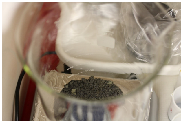
Figure 2.7: Uranium ore after ball-milling.
