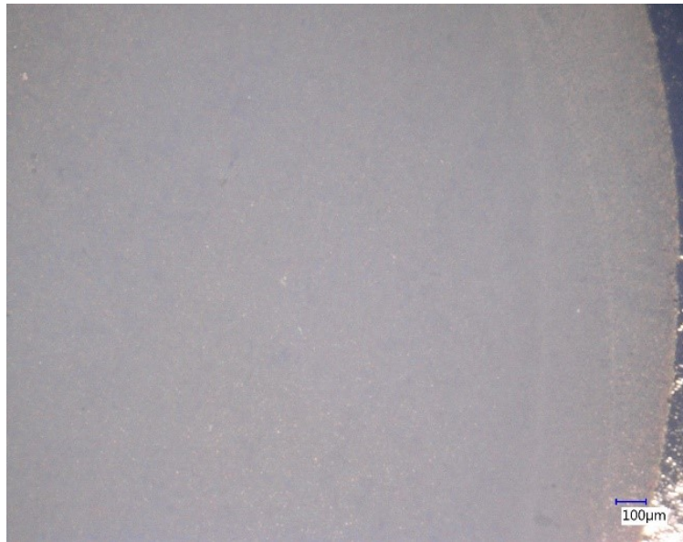
(b) ThO 2 ( 1100 \pm 66 \mu\text{g}/\text{cm}^2 ThO 2 ) on titanium. Faint circular arcs from inexact placement of the o-ring are visible, but with no loss of target quality at the edges.
