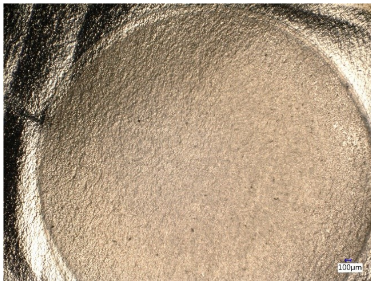
(b) Same target after igniting with a natural gas Bunsen burner, defects significantly reduced.
