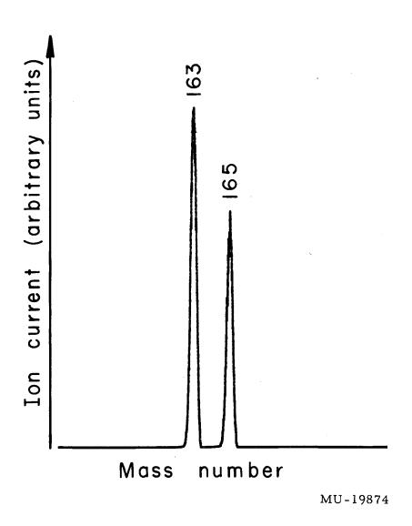
Fig. 1. Mass spectrum of the purified holmium fraction showing the long-lived 163 and stable 165 holmium isotopes.
