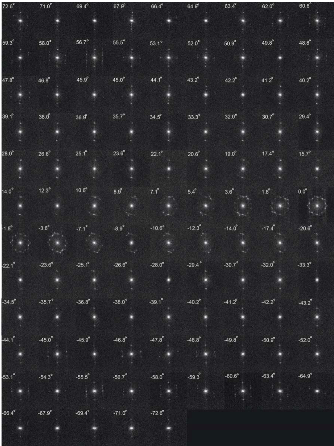
Supplementary Figure 2. Fourier transforms of the 104 projections (Supplementary Fig. 1), in which Bragg peaks are visible in most projections.
