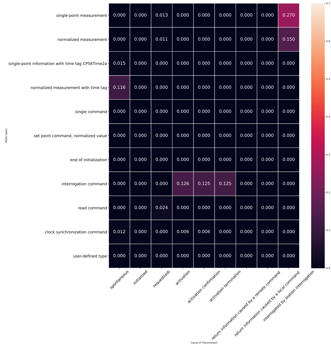
Figure 6.3: Distributions of transmission causes for I-format messages, the natural gas distribution network
