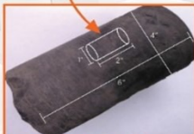
4x6-inch core from which 1x2-inch core plugs were drilled
