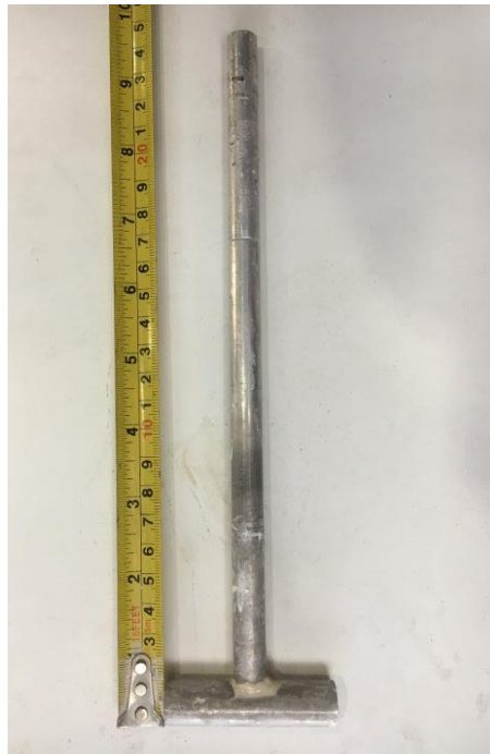
Figure 6.12: (a) T-bar dimensions, (b) T-bar photograph
