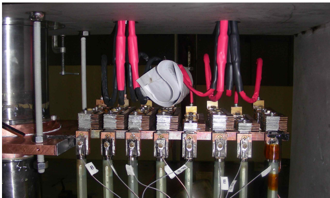
Fig. 2. The HTS and Copper Leads for the MICE Spectrometer Solenoid
