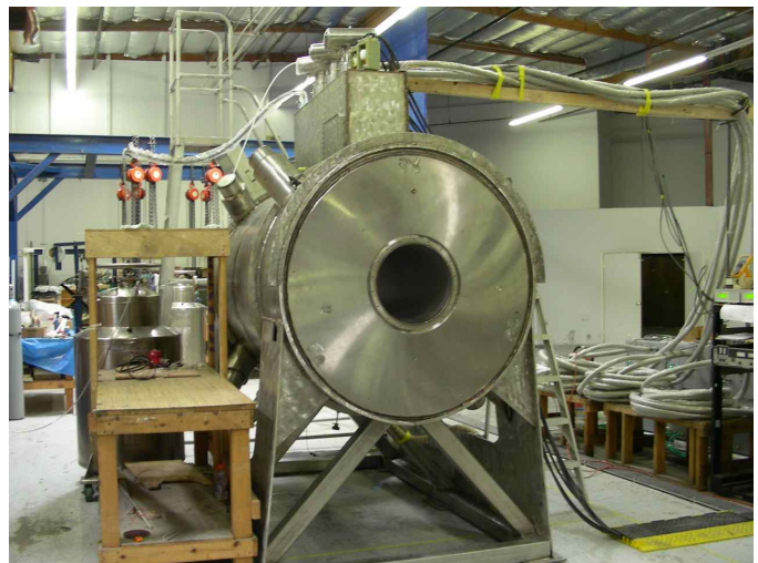
Fig. 3. Finished Spectrometer Solenoid 1 before the Magnet Cool-down
