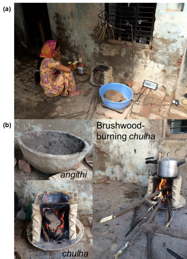
Figure 1. The field site and setup for cooking events. (a) The kitchen setup at the field site. (b) The stoves and fuels used in this study: angithi , dung-burning chulha , and brushwood-burning chulha .
