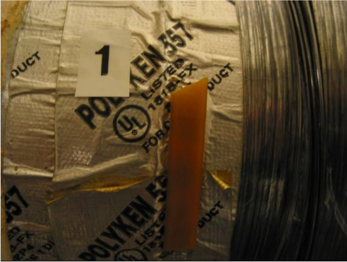
Figure A2. Sample 1. The second seal still has part of the nylon clamp in place. This shows the same characteristics as in Figure A1.
