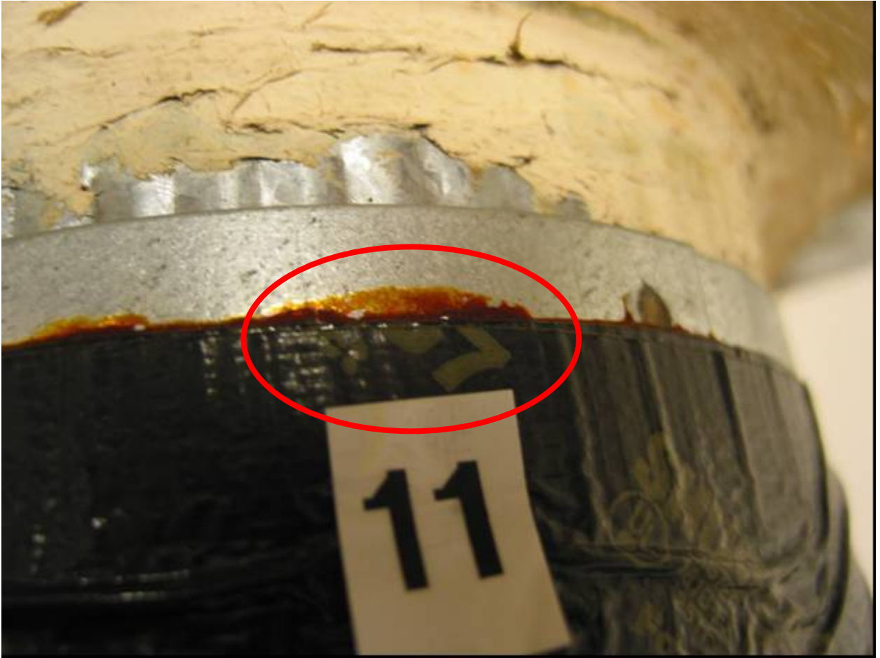
Figure A13. Sample 11. The adhesive has oozed out the edge of the tape.
