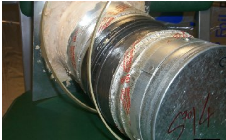
Figure 17 Failed Plastic Strapping On One Of The Flexible Core To Sheet Metal Collar Specimens After Four Months Of Aging
