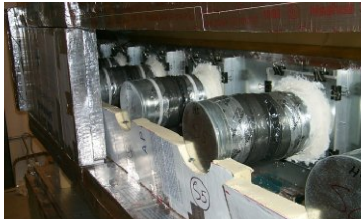
Figure 5 One Chamber Of The High Temperature Aging Test Apparatus
