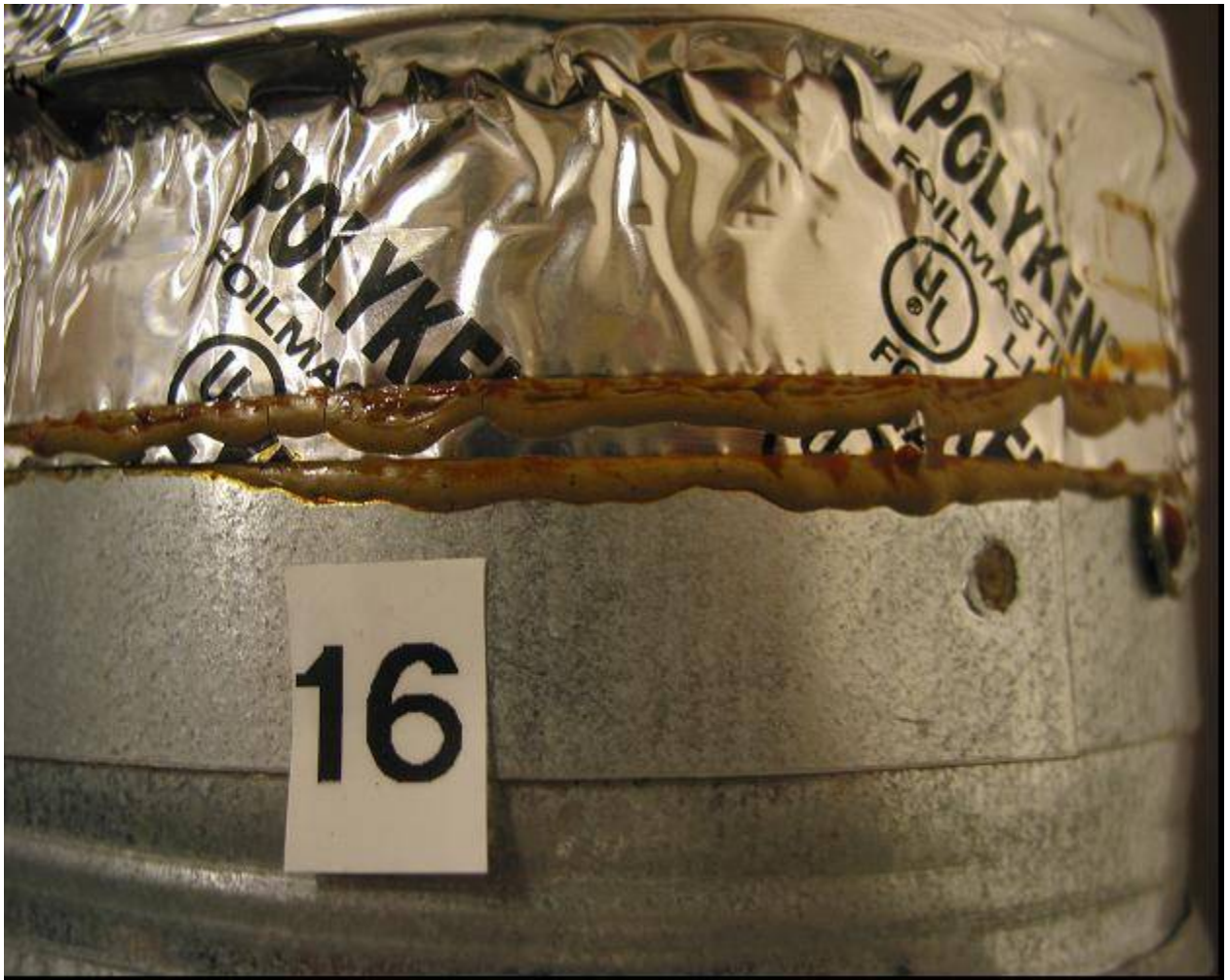
Figure A19. Sample 16. This sample shows oozing of the adhesive at the tape edges.
