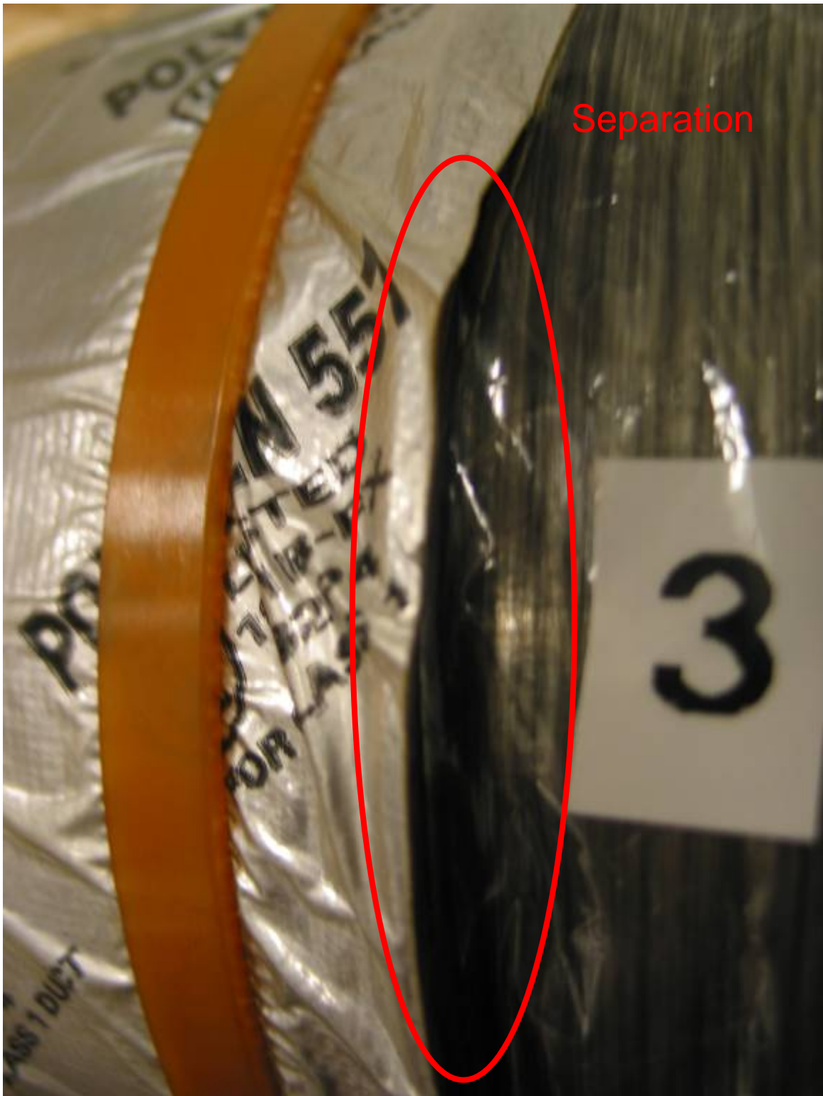
Figure A4. Sample 3. Tape has separated from the flex duct core at the tape edges
