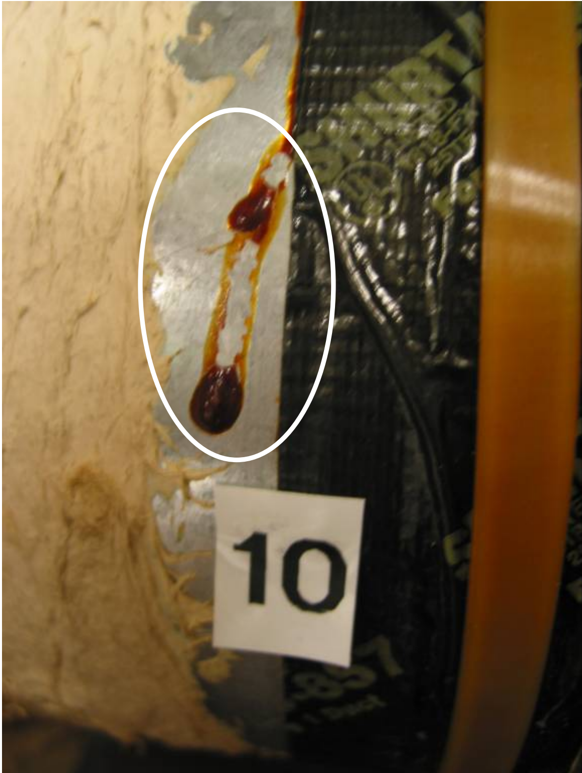
Figure A12. Sample 10. The adhesive has oozed out onto the surface of the duct.
