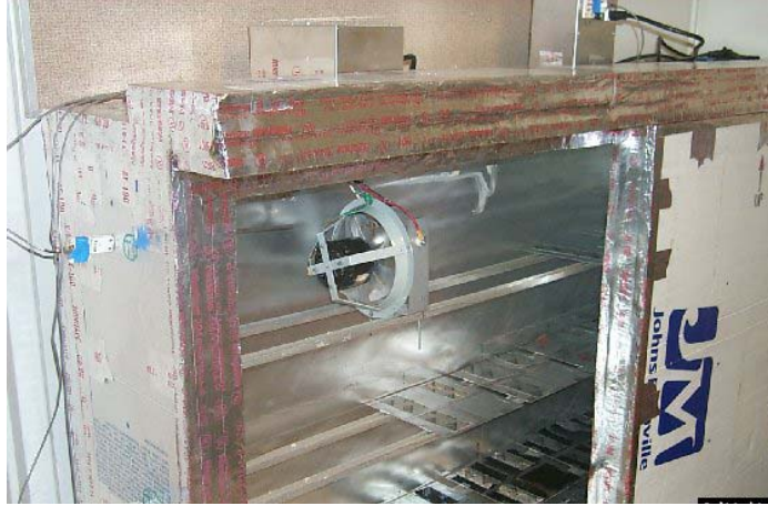
Figure 8 High Temperature Baking Apparatus
