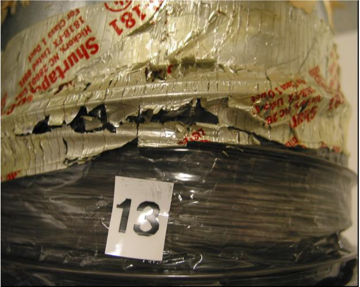
Figure A15. Sample 13. This sample shows cracking and disintegration of the tape
