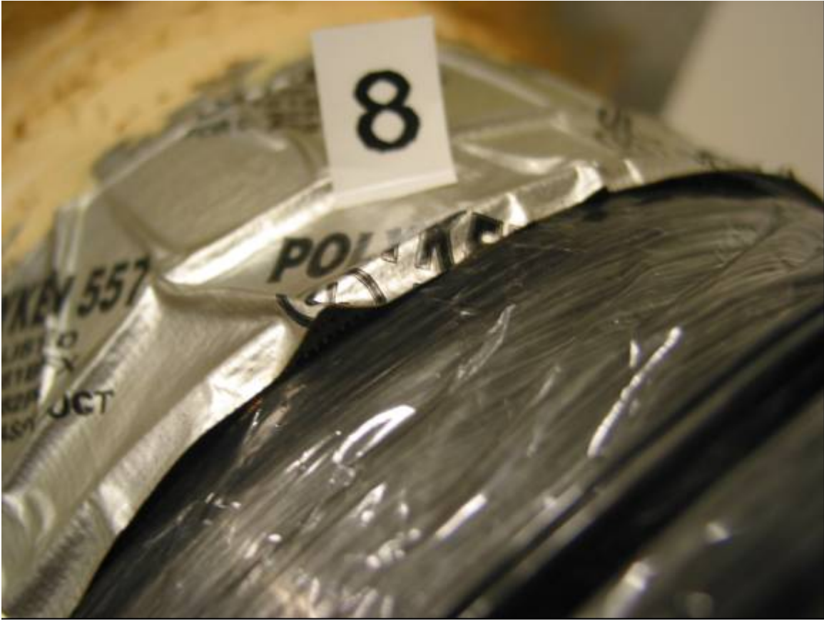
Figure A9. Sample 8. The edges of the tape are no longer stuck to the flex duct core.
