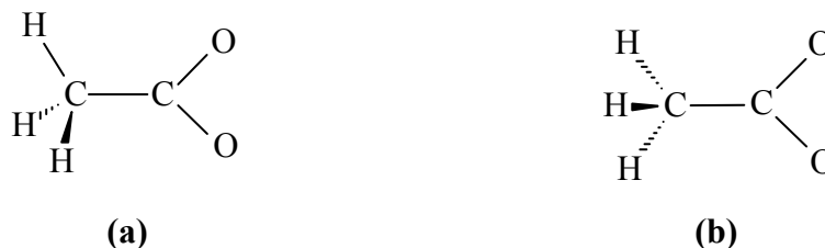
Figure 3-1: Structures of the CH 3 CO 2 radical. (a) One hydrogen atom lies in the plane of O-C-O group. (b) One hydrogen atom is in the plane bisecting O-C-O group.
