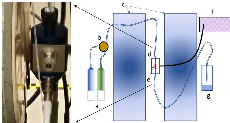
Figure 3. Generalized scheme for Flow Spin-trapping Experiments. Left side, photograph of spin trap column in front of EPR resonator. Right, instrument setup: a) Double syringe pump, b) mixer, c) EPR electromagnet, d) EPR resonator, e) spin trap column, f) UV lamp connected to resonator with flexible light pipe, g) solvent waste.
