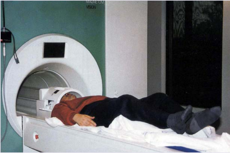
Figure 1 A subject is being prepared for a magnetic resonance examination. The subject lies in front of the magnetic resonance instrument on a movable bed. His head is encircled by an electronic device, which serves both to transmit low-energy radio frequency (RF) waves to hydrogen or phosphorus nuclei in the head and to receive the energy emitted from these nuclei. For the examination, the bed on which the subject lies is moved into the tunnel so that the magnet completely surrounds the subject's head. The magnetic field affects all nuclei in the body so that they will absorb and emit RF energy.
