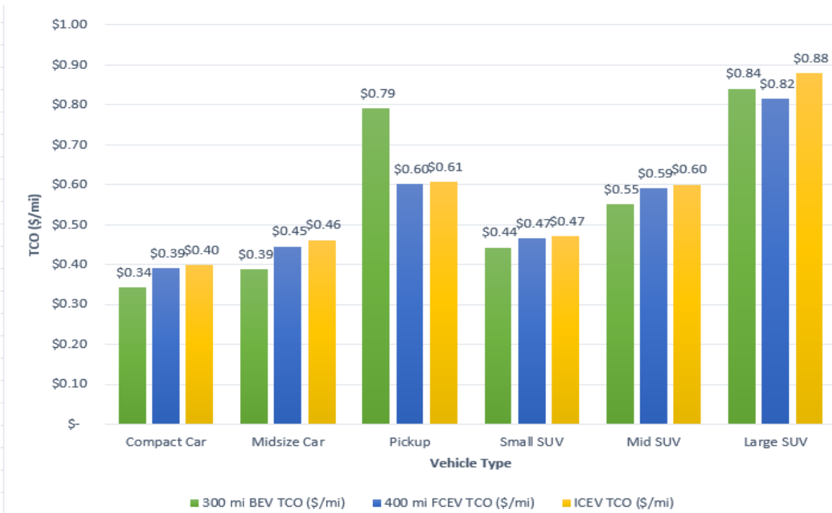
Figure ES-2: First (purchase) cost and TCO comparisons of electrified vehicles in 2030
