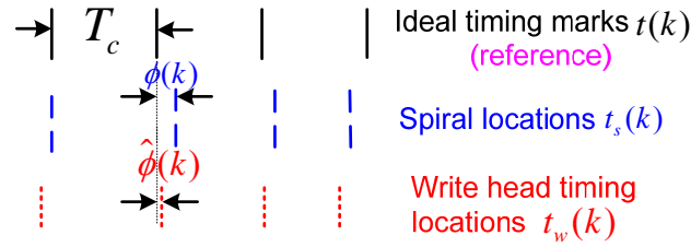
Figure 7.10: Illustration of read/write head timing locations in conventional PLL circuit
