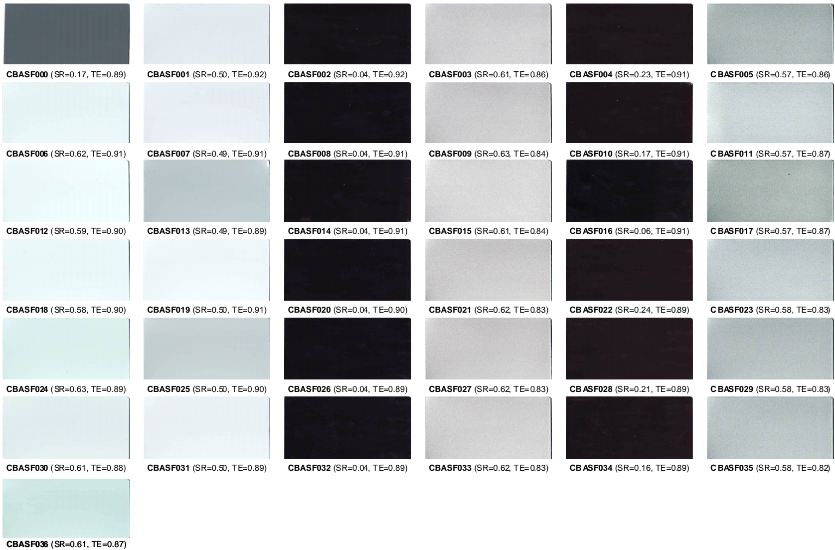
Figure 1. Sample set BASF1 includes one ecoat-only panel (CBASF000) and 36 primer/basecoat combinations (CBASF001-036). Each sample is labeled with its tracking code (CBASF nnn ), solar reflectance (SR) and thermal emittance (TE).
