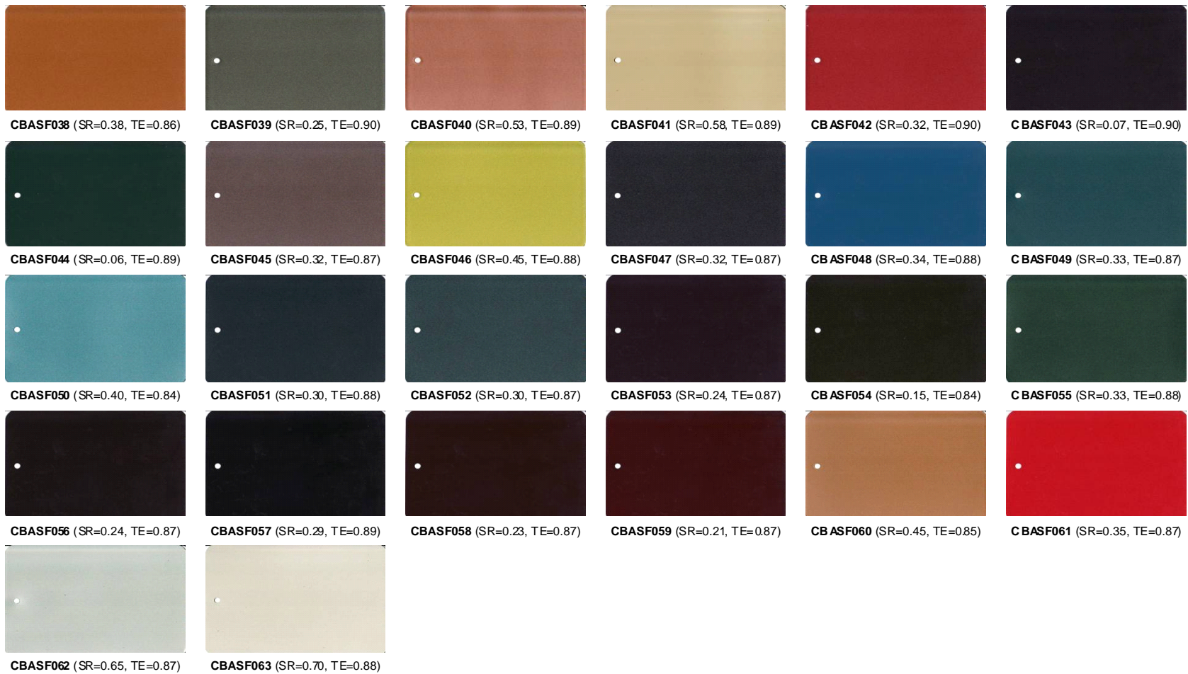
Figure 2. Sample set BASF2 includes 26 colors (CBASF038-063). Each sample is labeled with its tracking code (CBASF nnn ), solar reflectance (SR) and thermal emittance (TE).
