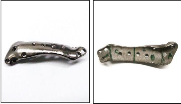
**FIGURE 3:** Additively manufactured Ti 6AL4V bone plate to correct radial deformity. The finished top surface (left) and the unfinished bottom surface (right) are shown.
