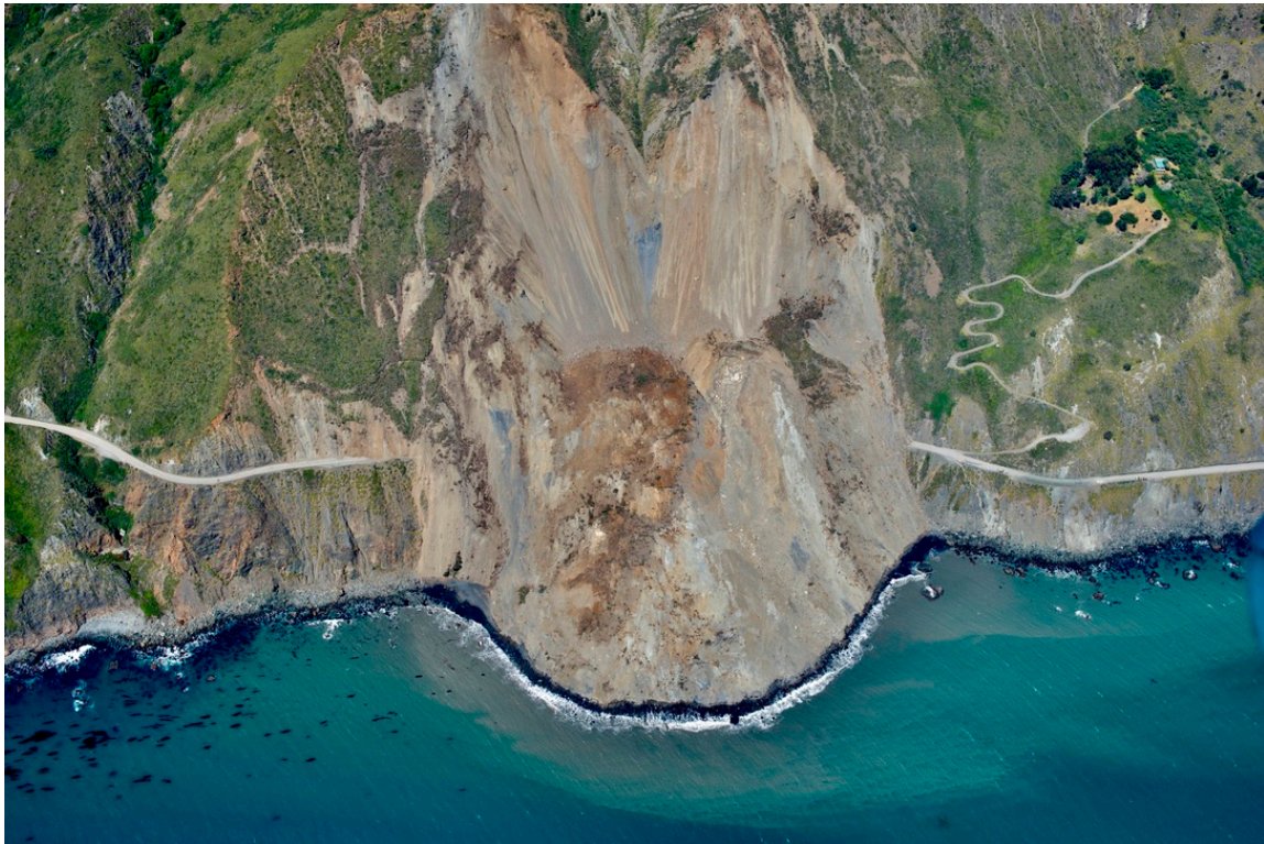
Figure 8. Steep mountainous coast in the Big Sur area of Central California with Mud Creek landslide (May 2017- Jon Warrick, U.S. Geological Survey).
