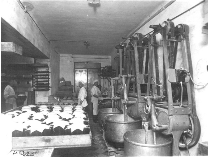
Mixers at an industrial baking plant in the early twentieth century, courtesy of thefreshloaf.com
