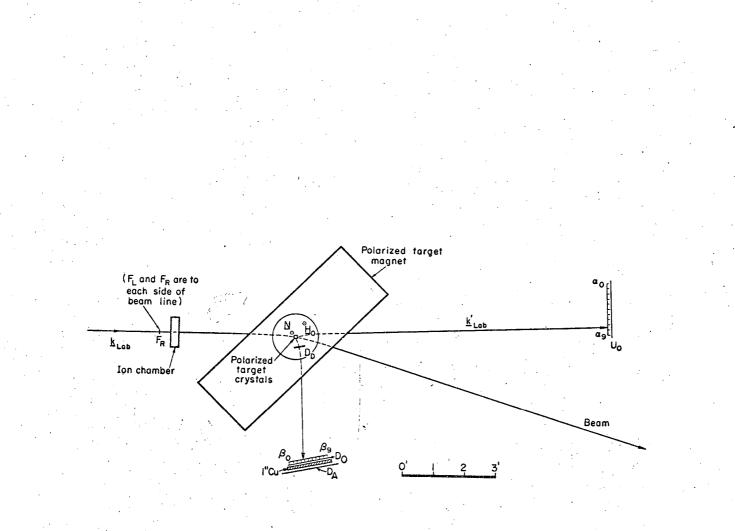
Fig. 6. Arrangement of the scintillation counters. The counter dimensions were:
